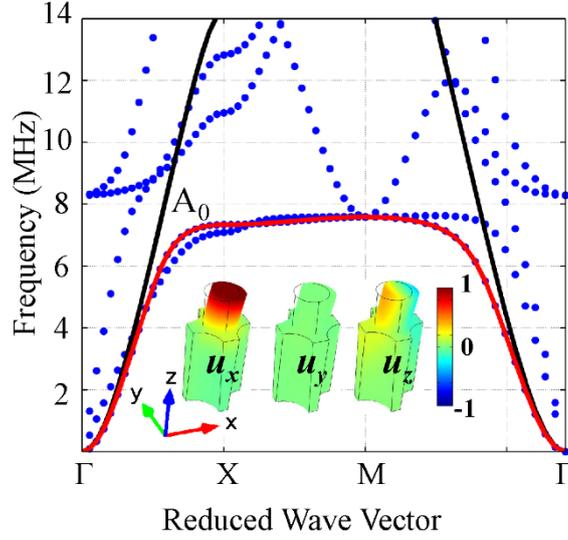
Figure 3.6. Band structure (dotted curves) of the trampoline GRIN structure along the central layer of the acoustic lens. The  $A_0$  band is highlighted by the overlapping red line while the black line indicates the  $A_0$  band along the central layer without pillars. Inset shows the normalized modal displacements of the  $A_0$  mode at the X point in the Brillouin zone. This figure is reproduced from Ref. [141].
