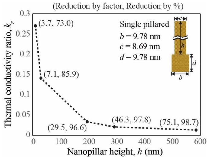
Figure 6.7: Thermal conductivity ratio  $k_r$  versus nanopillar height for a membrane with a thickness of 9.78 nm. Numbers in parenthesis indicate the thermal conductivity reduction due to addition of the nanopillar, given as a
