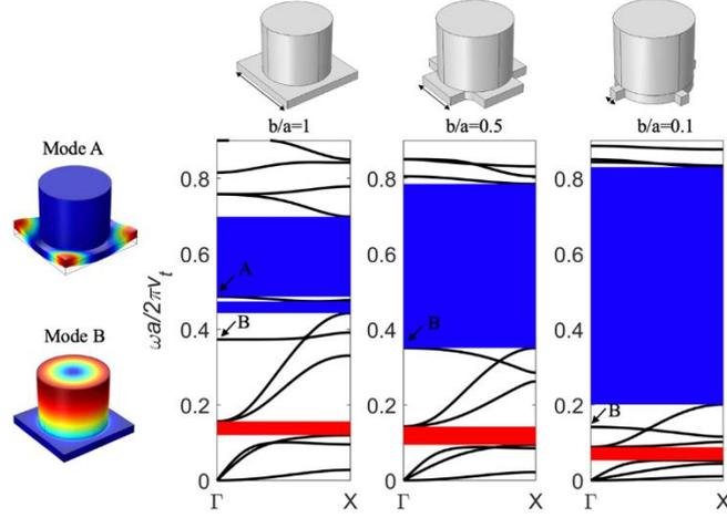
Figure 3.3. Dispersion for pillared phononic crystals connected by thin bars with the bar's width as  $b/a=1$  (left), 0.5 (middle) and 0.1(right). The Bragg and hybridization band gaps are respectively marked in blue and red. The geometries of the unit cells are displayed on top of each dispersion curve, respectively. The eigen modes of band A and B at the  $\Gamma$  point are also represented at the left. This figure is adapted from Ref. [61].
