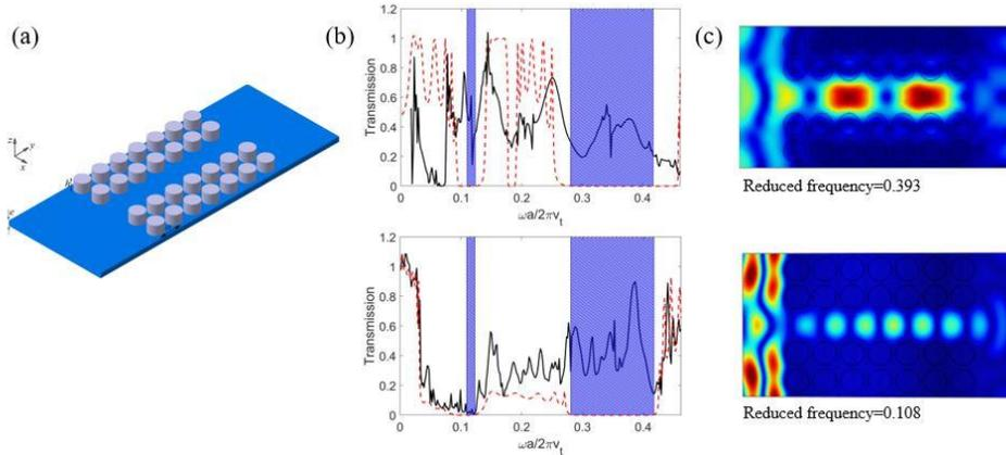
Figure 2.8. (a) Schematic view of a line-defect waveguide; (b)  $S_0$  Lamb wave excitation (upper) and  $A_0$  Lamb wave excitation (lower) transmission through the waveguide (black solid lines) and through the perfect (red dashed
