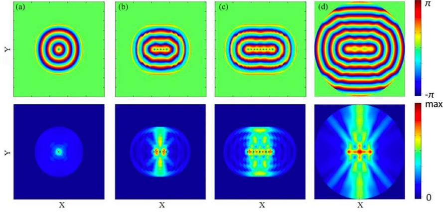
Figure 4.3. Phase (upper panel) and amplitude (lower panel) of the scattered wave for (a) a single pillar at a compressional mode; (b) adding five single sources with a inter distance of  $200 \mu\text{m}$  numerically; (c) similar as (b) but for nine single sources; (d) one real line of nine pillars inter distance as  $200 \mu\text{m}$ . This figure is reproduced from Ref. [90].
