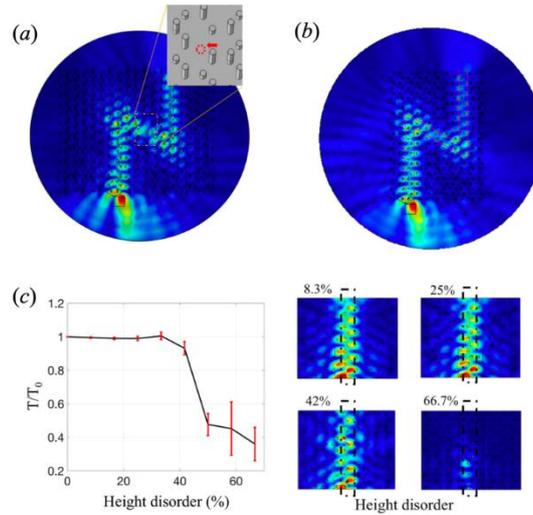
Figure 5.2. (a) Topologically protected zigzag interface state against a defect. (b) The same zigzag state against a minimized bulk size with only one hexagon unit beside the interface. (c) In the left panel, transmission property versus height disorder level of the pillars of the interface; in the right panel, the flexural wave propagation field for four selected height disorders. This figure is adapted from Ref. [151].
