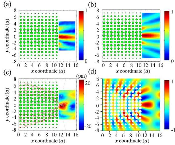
Figure. 3.7. (a) Experimental and (b) numerical distribution of the normalized maximum  $u_z$  behind the acoustic lens at the X point in the Brillouin zone (7.2 MHz), together with (c) experimental and (d) numerical snapshots of the near field focusing at 7.2 MHz. (c) The gray solid lines and the red dashed lines are for the ray trajectories with  $|k_y| < k_B$  and  $|k_y| > k_B$ , respectively. This figure is reproduced from Ref. [141].
