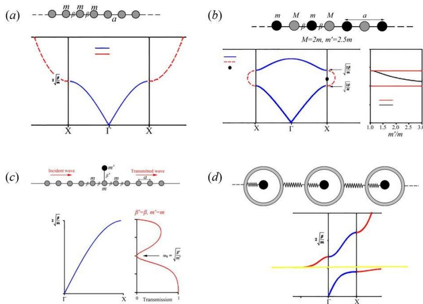
Figure 2.1. Mass-spring models and corresponding dispersions: (a) a linear monoatomic chain made of identical atoms; (b) a biatomic linear chain comprising two different atom types; (c) a side atom is attached to monoatomic linear chain; (d) a periodic array of side atoms is attached to the linear chain to form a locally resonant periodic chain.
