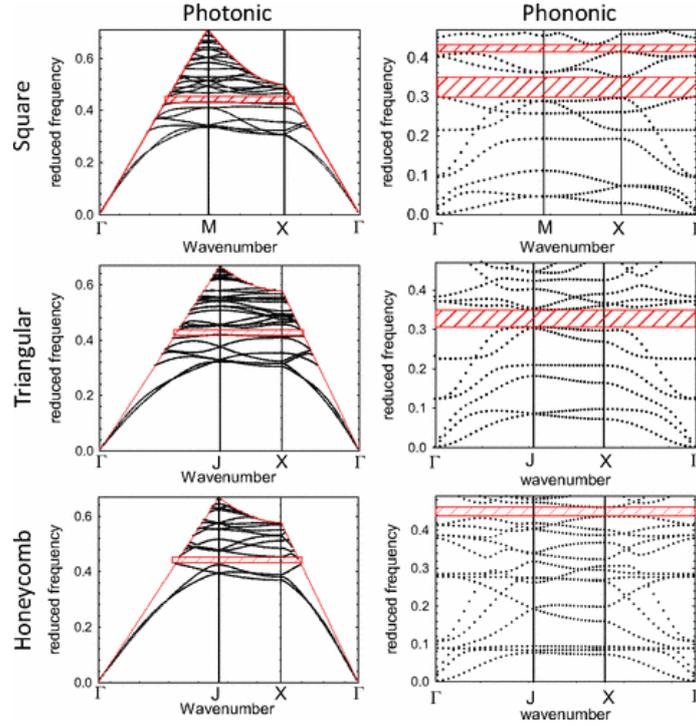
Figure 2.14. Photonic (left) and phononic (right) dispersions curves calculated for (a) a square array with the set of parameters  $e_{SiO_2}/a = 0.2$ ,  $h_{Si}/a = 0.8$  and  $f = 0.4$ , (b) a triangular array with the set of parameters  $e_{SiO_2}/a = 0.5$ ,  $h_{Si}/a = 0.8$  and  $f = 0.5$  and (c) a honeycomb array with the set of parameters  $e_{SiO_2}/a = 0.4$ ,  $h_{Si}/a = 0.7$  and  $f = 0.3$ . This figure is reproduced from Ref. [45].
