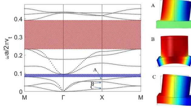
Figure 2.3. Dispersion curves for the following pillared plate: steel pillar's radius  $r/a=0.42$ , pillar's height  $h/a=0.6$  and the silicon plate's thickness  $e/a=0.1$ . The red and blue dash zones indicate Bragg and local-resonance hybridization band gaps, respectively. Eigenmodes corresponding to the three points A, B and C at X are displayed at the right. This figure is based on results from Ref. [19].
