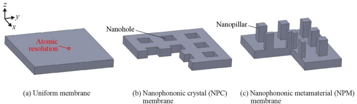
Figure 6.1: Three silicon membrane configurations: (a) Uniform, (b) nanophononic crystal, and (c) nanophononic metamaterial.
