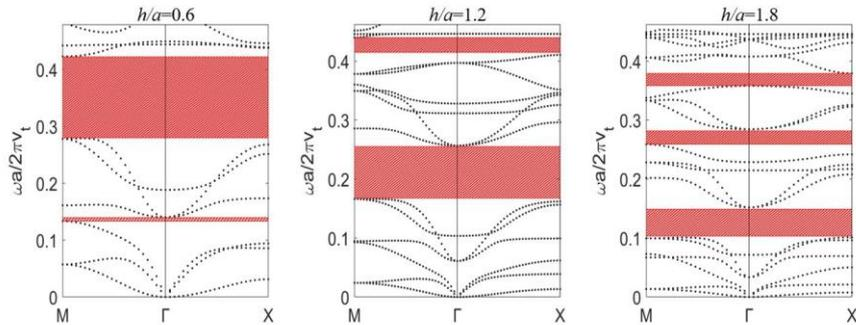
Fig. 2.4. Evolution of the band structure for different values of the height of the pillar: (left)  $h/a = 0.6$ , (middle)  $h/a = 1.2$  and (right)  $h/a = 1.8$ . The other geometrical parameters are  $e/a = 0.2$  and  $r/a=0.42$ . This figure is based on results from Ref. [19].
