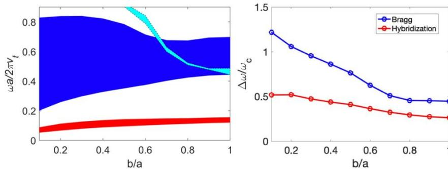
Figure 3.4. (Left) Evolution of the Bragg (blue) and hybridization (red) band gaps as a function of bar's width  $b/a$ . The cyan color represents band A, a torsion mode. (Right) Relative size of band gaps as a function of bar's width  $b/a$ . This figure partially includes results from Ref. [61].
