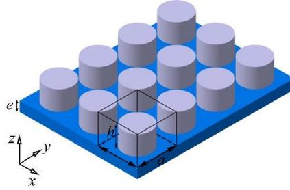
Figure 2.2. Geometry of a phononic crystal plate consisting of periodic pillars deposited on a thin plate. In the present section, the plate's thickness is denoted by  $e$ , and the height of the pillars by  $h$ .
