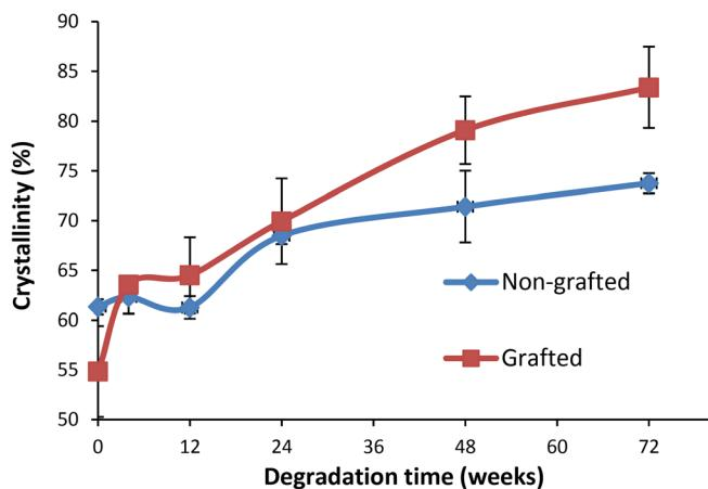
**FIGURE 5** Crystallinity rate of G and NG samples degraded in PBS at 37°C for 72 weeks [Color figure can be viewed at [wileyonlinelibrary.com](http://wileyonlinelibrary.com)]
