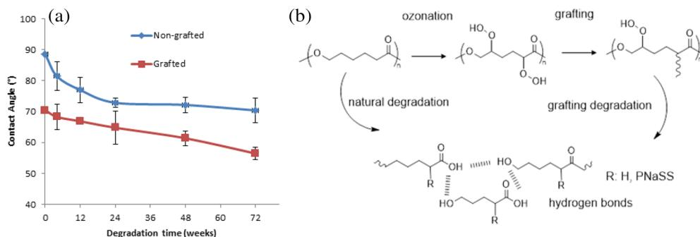
**FIGURE 2** (a) Water contact angle measured by the sessile drop method on G and NG medical-grade poly( $\epsilon$ -caprolactone) (PCL) samples and its evolution with degradation time. (b) Scheme of hydrolytic degradation of NG PCL (natural degradation) and G PCL (grafting degradation) [Color figure can be viewed at [wileyonlinelibrary.com](http://wileyonlinelibrary.com)]
