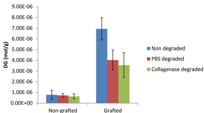
**FIGURE 13** Poly(sodium styrene sulfonate) (pNaSS) grafting density over medical-grade poly( $\epsilon$ -caprolactone) (PCL) before and after 6 months of degradation in PBS or 50 mg/ml collagenase solution at 37°C. virgin PCL samples were used as control of non-specific absorption [Color figure can be viewed at [wileyonlinelibrary.com](http://wileyonlinelibrary.com)]
