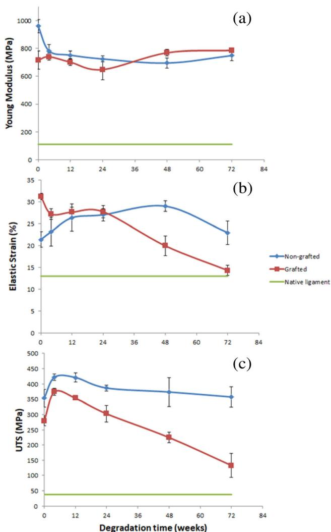
**FIGURE 6** Monitoring of Young's modulus (a), elastic deformation (b) and ultimate tensile strength (c) evolution of G and NG samples degraded in PBS at 37°C [Color figure can be viewed at [wileyonlinelibrary.com](http://wileyonlinelibrary.com)]
