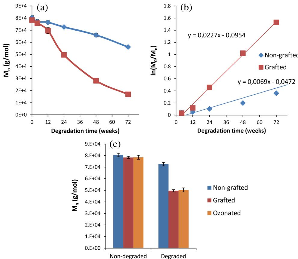
**FIGURE 4** Number molecular weight evolution (a), modified Arrhenius plot for half-life molecular weight reduction calculation (b) and number molecular weight variation of G and NG samples compared to ozonated films after 24 weeks of degradation at 37°C in PBS (c) [Color figure can be viewed at [wileyonlinelibrary.com](http://wileyonlinelibrary.com)]
