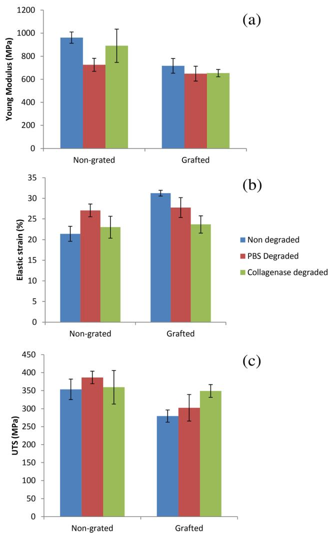
**FIGURE 11** Young modulus, elastic deformation and ultimate tensile strength of poly( $\epsilon$ -caprolactone) (PCL) fibers after 24 weeks of degradation in different degradations environment [Color figure can be viewed at [wileyonlinelibrary.com](http://wileyonlinelibrary.com)]
