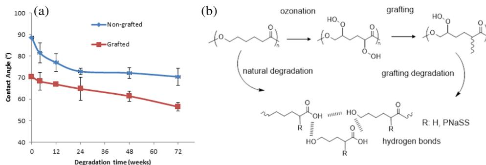
**FIGURE 2** (a) Water contact angle measured by the sessile drop method on G and NG medical-grade poly( $\epsilon$ -caprolactone) (PCL) samples and its evolution with degradation time. (b) Scheme of hydrolytic degradation of NG PCL (natural degradation) and G PCL (grafting degradation) [Color figure can be viewed at wileyonlinelibrary.com]
