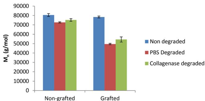
**FIGURE 10** Number molecular weight of G and NG samples degraded in PBS and collagenase solution for 24 weeks at  $37^\circ\text{C}$  the  $M_n$  reduction was statically smaller in samples G in collagenase solution ( $p < 0.05$ ) [Color figure can be viewed at wileyonlinelibrary.com]
