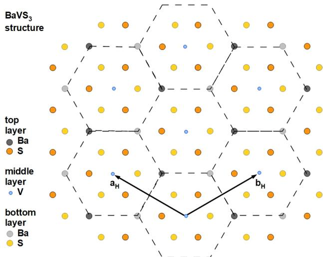
Figure 1. Room temperature hexagonal structure of  $\text{BaVS}_3$ , seen along the  $c$  axis, presenting a top  $\text{BaS}_3$  plane, middle V-layer and a bottom  $\text{BaS}_3$  layer.  $a_H$ ,  $b_H$  are for the hexagonal unit cell wave vectors. According to recent structural refinements<sup>21</sup> the Ba/S and V subsystems are not adjusted in terms of space group at RT.
