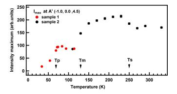
Figure 3. Temperature dependence of the DS intensity at the A' point. It is derived from two distinct measurements, performed on two different samples. Sample 1 (red points) is a pure BaVS<sub>3</sub>, studied in this work. Black points are revisited data from a slightly Al-doped sample, studied previously<sup>39</sup>. The intensity of the second measurements is normalized in order to obtain the same intensity at a common temperature of about 110 K.
