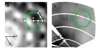
Figure 9. (a) Calculated TDS intensity in the (h, k, 3.5) plane, corresponding to the Cmc2<sub>1</sub> space group, indexed in hexagonal settings. The green hexagon, white dotted lines and particular points A'<sub>1</sub>, L', A'<sub>2</sub>, A, indicate the portion of the momentum space where the phonon analysis was performed. (b) Reconstruction of the measured (h, k, 3.5) plane at 114 K. The green hexagon indicates the same region as in (a).
