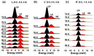
Figure 6. IXS scans at two satellite positions, (a) L point at (0, -0.5, 4.5), (b) L' point at (0.5, 0.5, 4.5) and (c) at the hexagon-diffuse corner, A' point at (0, -1, 4.5). They are fitted with three structures: a central peak (CP, black), a low energy phonon (LE, red) and a high energy phonon (HE, yellow).
