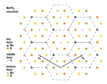
Figure 1. Room temperature hexagonal structure of BaVS<sub>3</sub>, seen along the c axis, presenting a top BaS<sub>3</sub> plane, middle V-layer and a bottom BaS<sub>3</sub> layer.  $a_H$ ,  $b_H$  are for the hexagonal unit cell wave vectors. According to recent structural refinements<sup>21</sup> the Ba/S and V subsystems are not adjusted in terms of space group at RT.
