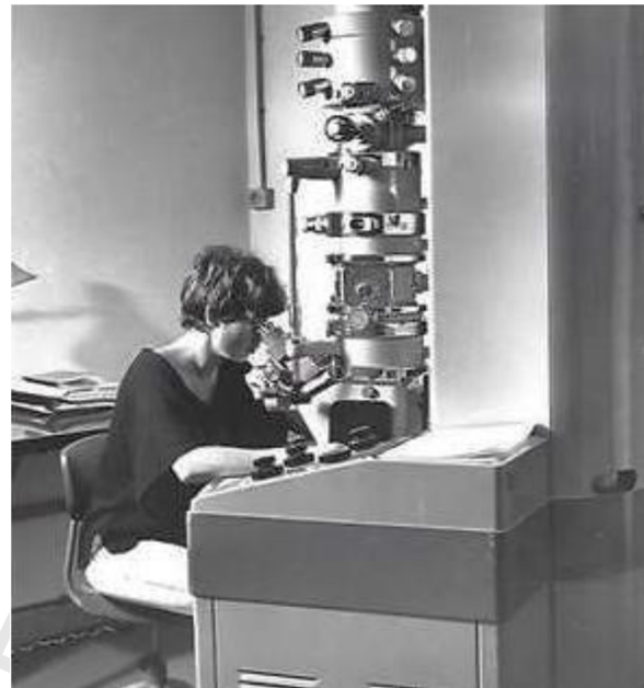
Fig. 1. 1975. The first transmission electron microscope (Hitachi HU11A) in place at the Arago Laboratory (the first in a french marine station). Seating and working Marie-Odile Soyer-Gobillard. (©J. Lecomte, Bibliothèque du Laboratoire Arago/Sorbonne Université).
