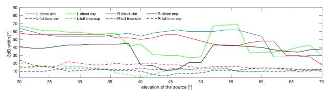
Figure 12. -3dB width of the focusing functions for the direct and full-time correlations and left (L) and right (R) receivers when the input signal is a linear chirp as in Figure 11 for simulations and a narrower-band linear chirp for experimental case.
