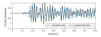
Figure 8. Comparison of the experimentally recorded (black) and numerically simulated (blue) acceleration, for source elevation of 82°. The amplitude of the reverberated part of the experimental data is scaled as in Figure 7b.
