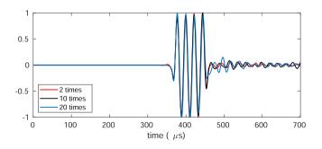
Figure A.2. Comparison of the signals for a slice with 3 different resolutions: 0.22 mm (red), 1.1 mm (black), 2.2 mm (red).
