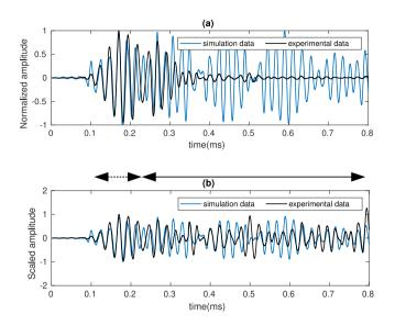
Figure 7. Comparison of the acceleration signals recorded in the experiment (black) and the simulation (blue) for a source elevation of  $25^{\circ}$  (a) with the normalized amplitude and (b) with the scaled normalized amplitude. Dashed and solid arrows mark the direct arrival and coda windows, respectively.
