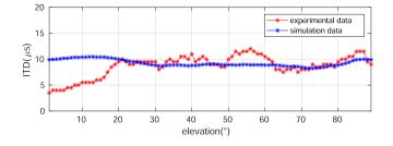
Figure 9. Comparison of the time difference between the signals received at the left and right receivers obtained from the experimental (red) and simulation (blue) data. Uncertainty of the experimental values is around 5  $\mu$ s.
