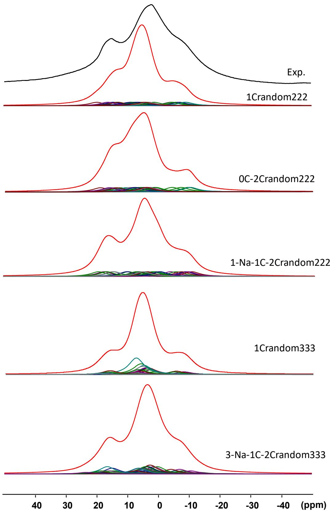
**Figure S5.**  $^{11}\text{B}$  experimental solid-state NMR spectrum of  $\text{NaB}_5\text{C}$ -related sodium carbaboride powder and calculated spectra of the different models proposed replacing quadrupolar lineshapes by broadened Gaussian lines.
