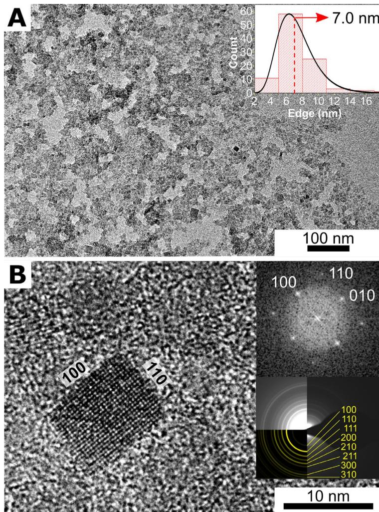
**Figure 2.** (A) TEM and (B) HRTEM images of NaB<sub>5</sub>C-related sodium carbaboride nanocrystals. The corresponding size distribution is shown as inset in (A). The Fast Fourier Transform (FFT) of image (B) is shown as insert, together with the SAED pattern. They are fully indexed along the NaB<sub>5</sub>C structure.
