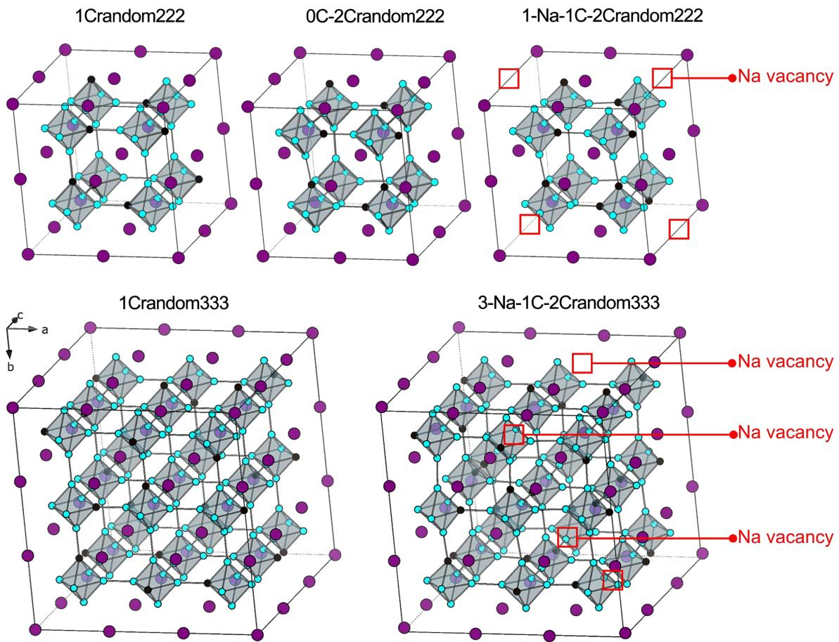
**Figure 5.** Structural models used to calculate the  $^{11}\text{B}$  NMR spectra of sodium carbaborides.
