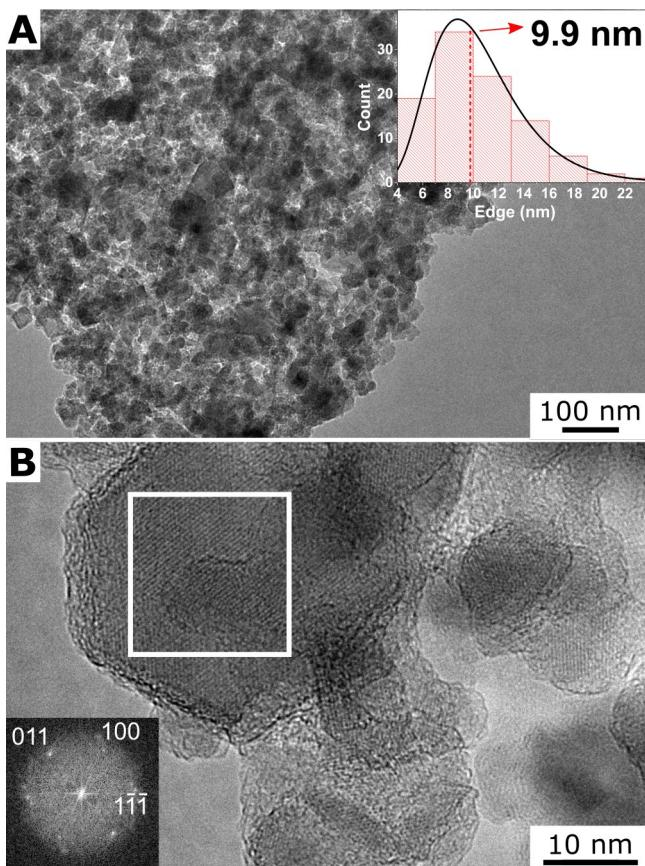
**Figure 7.** (A) TEM and (B) HRTEM images of boron carbide nanocrystals obtained by the decomposition of molten salt-derived sodium carbaboride nanocrystals. The inset in A shows the size distribution fitted with a lognormal function. The inset in B is a Fast Fourier Transform of the region marked with a white square. The reflexions are indexed along the rhombohedral boron carbide structure.
