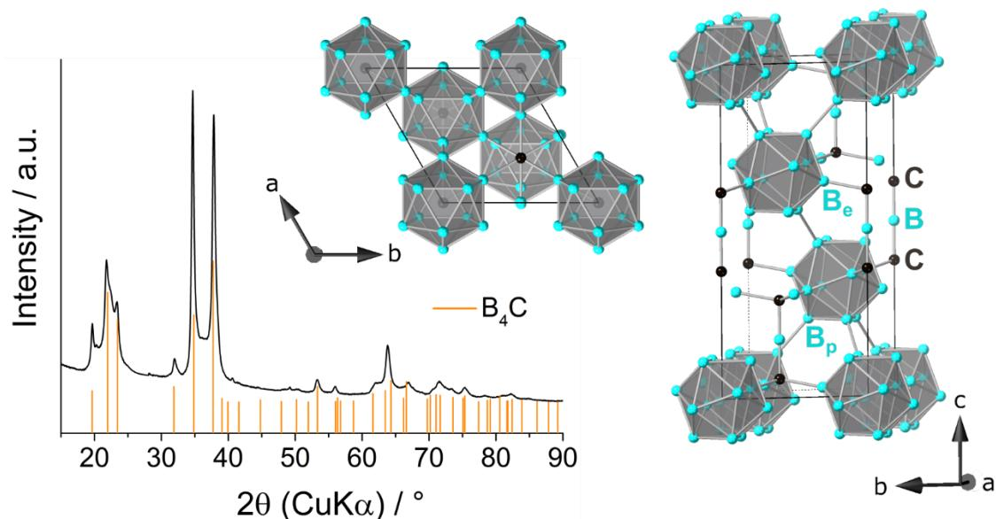
**Figure 6.** Powder XRD pattern of the powder obtained after calcination of sodium carbaboride nanocrystals. The reference pattern corresponds to rhombohedral B<sub>4</sub>C-type boron carbide. Two different views of a corresponding ideal crystal structure are displayed.
