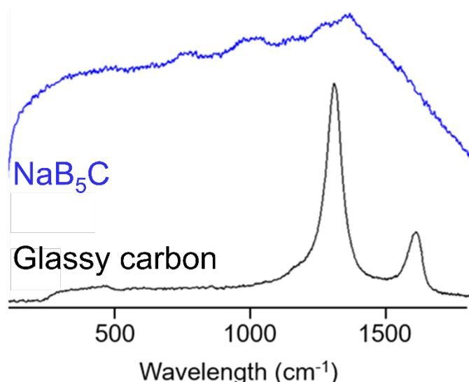
**Figure S2.** Raman spectra of sodium borocarbide nanocrystals (blue). The spectrum of glassy carbon is given as a reference (black), showing the two typical bands of disordered carbon with graphitic domains.
