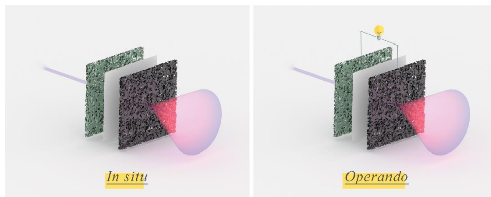
Figure 1. Scheme of in situ vs. operando experiments. Operando requires that the cycling is continuously performed and not stopped during the structural characterization.
