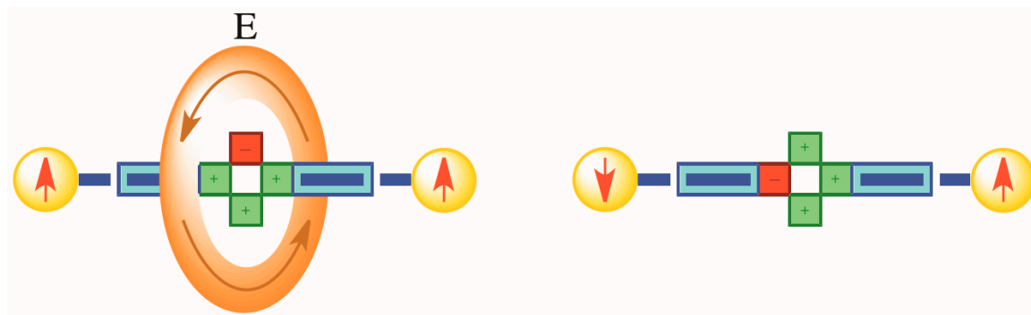
Figure 8. Illustration of the rectifying behavior in a molecular magnetic switch showing the inversion of the spin alignment from parallel to antiparallel induced by an external applied electric field. Adapted with permission from Castellano et al. (reprinted with permission from [100], American Chemical Society, 2015).
