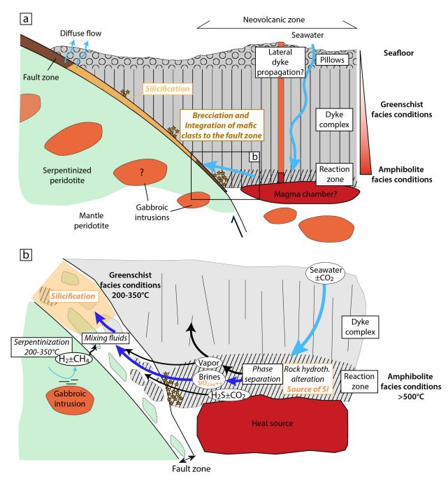
**Figure 12**: Schematic interpretation of fluid circulation along the 13°20'N OCC. (a) The 1518 hangingwall corresponds to a section of upper crust while the footwall progressively exhumes
