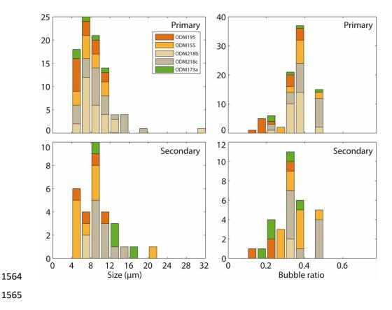
Figure S2: Size distribution (left) and bubble/inclusion volumetric ratio (right) histograms for primary (top)
