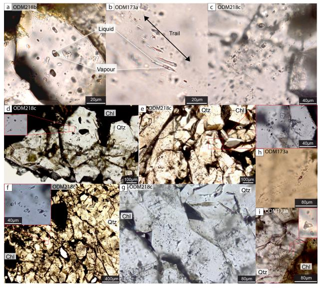
Figure 4: Microphotographs of representative two-phase (liquid and vapor) fluid inclusions in
