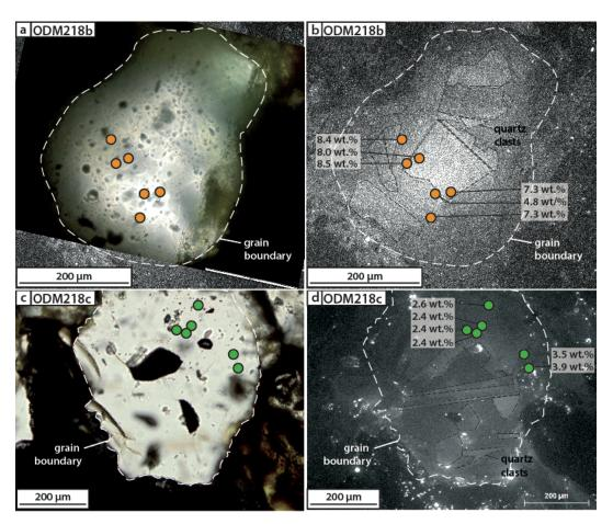
Figure 7: Distribution of measured fluid inclusions in quartz grains from ODM218b (a and b,
