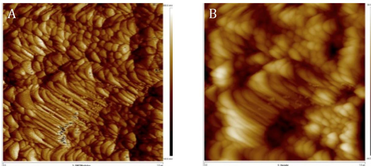
**Figure 4:** AFM imaging of a control titanium plate (1 μm scale)
