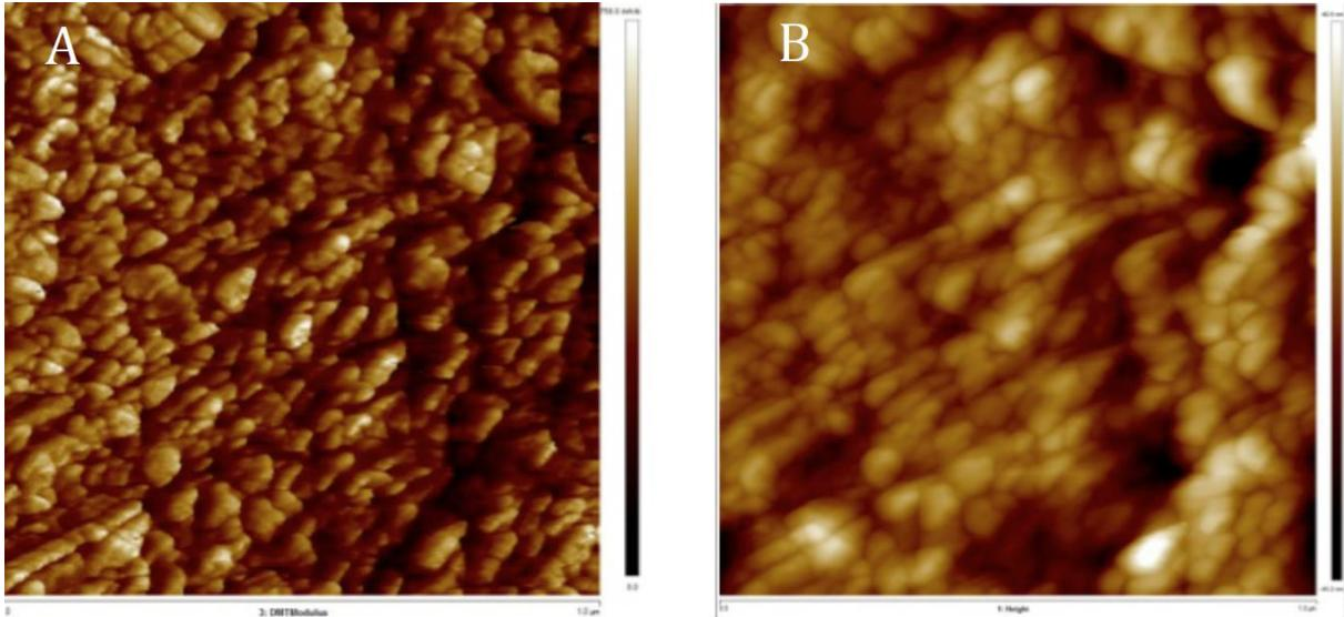
339 **Figure 5:** AFM imaging of grated plates spin-coated with Q-PVP-4days (1 $\mu$ m scale).
