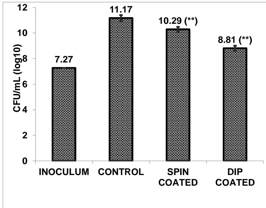
**Figure 11:** *In vitro* growth inhibition (24 hours) in rich medium (BHI) at 37°C. Inoculum: n=1 ; Control: n=9 ; Spin-coated: n=9 ; Dip-coated: n=9 ; All data are represented as mean ± standard error. All treated plates showed statistically significant differences in bacteriological count values compared with control (P<0.01).
