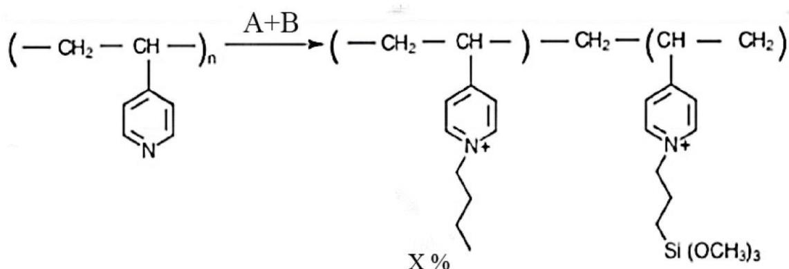
49 **Figure 1.** Quaternized polyvinylpyridine polymer synthesis
