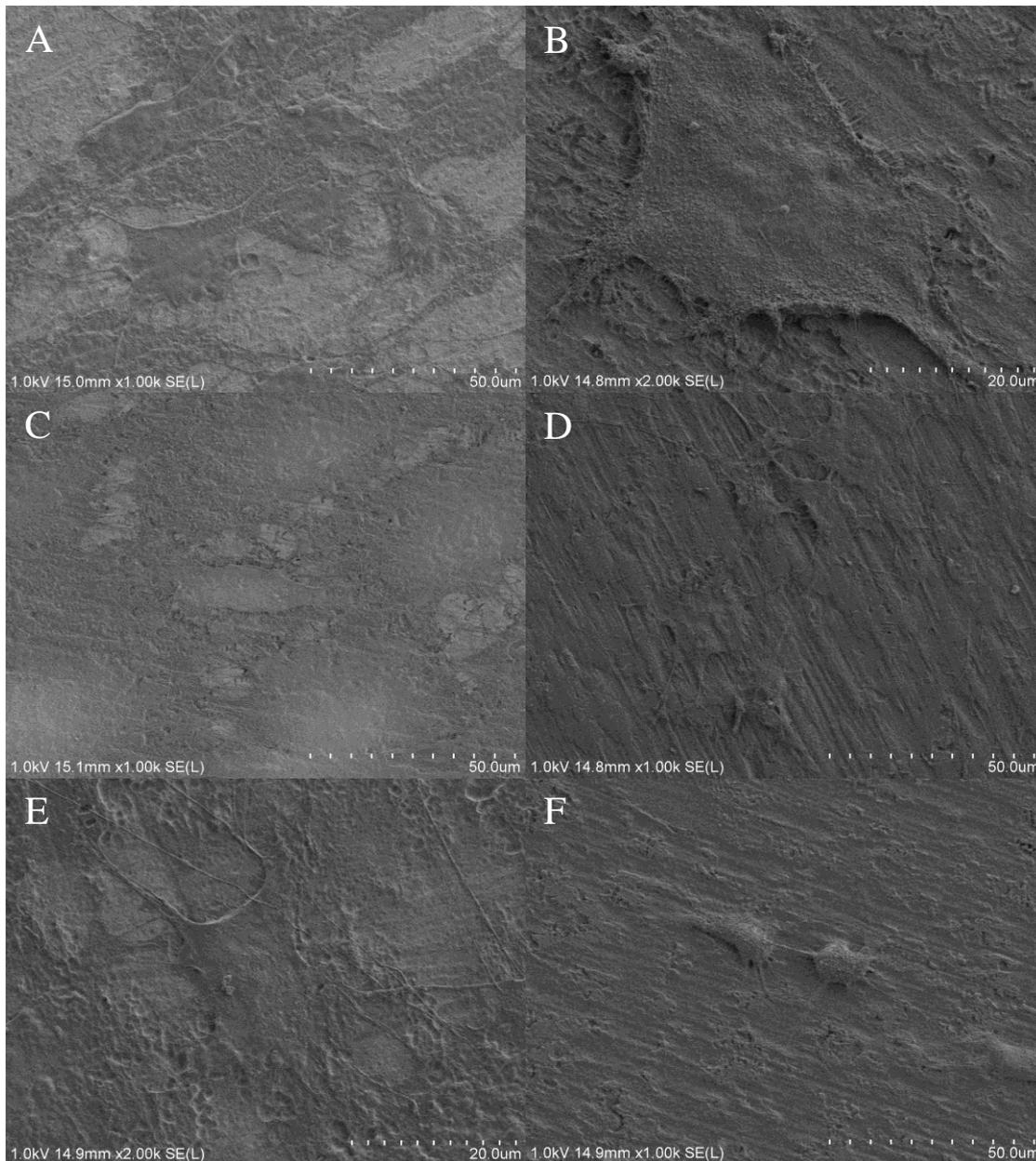
435 **Figure 9:** SEM-FEG imaging displaying gradual adherence decrease of MC3T3 cells on surfaces of
