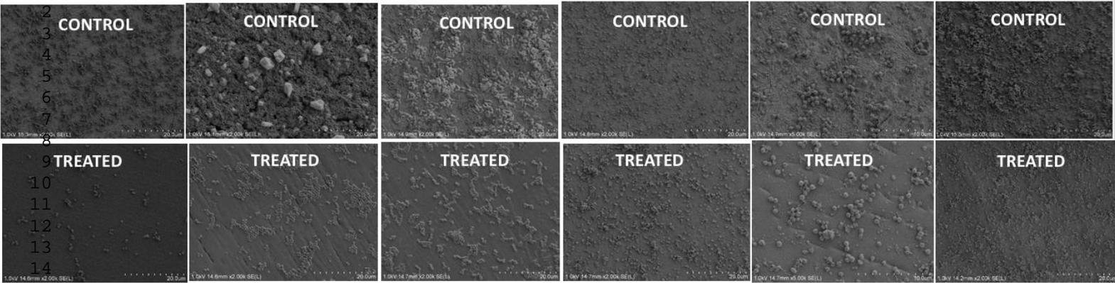
**Figure 12: MRSA biofilm growth on Q-PVP-4 days dip-coated surfaces vs control.**
