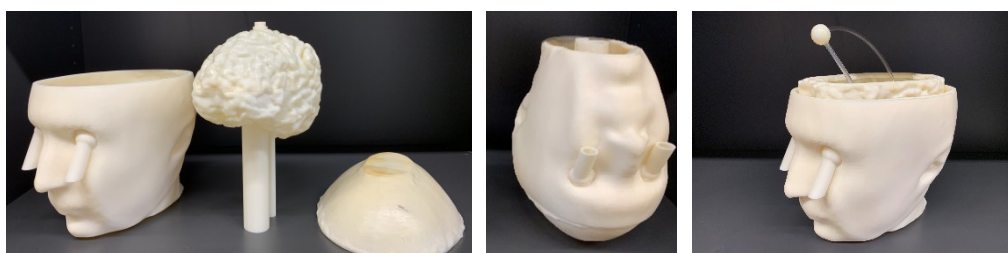
Figure 4. Upside down head phantom including the complex brain and an extra cavity as a muscle container. The stroke and the connected pipes are designed in a way to pass through the cylinders which are connected to the brain cavity and can be fixed in a random location inside of it.
