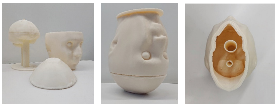
Figure 3. Upside-down configuration of the head phantom including the simple brain cavity.
