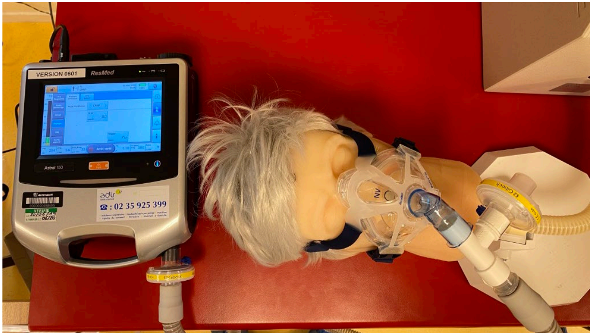
e-Figure 1: 3D-printed head model with setup 4 test.
