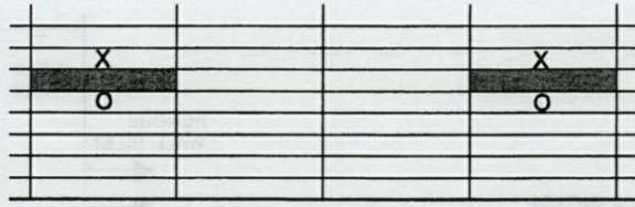
Fig. 2. – Side view of the first 8 cells above the bottom in the refined computational mesh (cell size 0.25 \times 0.25 \times 0.036 mm), showing locations of 2 pairs of sinks (×) and sources (○), separated by cell (cross-hatched) with impermeable horizontal faces.
