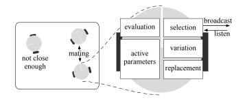
Fig. 1. Principle of embodied evolution algorithms. The robotic agent sends and receives parameters of a policy function, and uses a evolutionary algorithm to improve it own active parameters.
