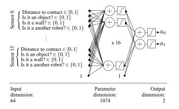
Fig. 4. Architecture of the policy function. Each sensor gives information about the distance to obstacle and the type of object detected, if any. The architecture represented here is a multi-layered Perceptron, used for the experiments. It has 64 dimensions as input, a hidden layer of 16 dimensions plus a bias term for each layer. The action dimension is 2. The total number of parameters is 1074.
