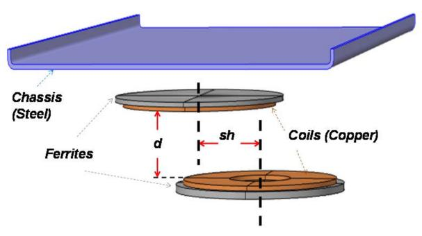
Figure 2. 3D structure of an ICT with shielding and a simple EV chassis, [52].
