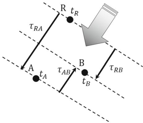
**Fig. 8** Closure delay defined by the difference in arrival time of an identical wavefront from a radio source at all three stations. A plane wavefront represents the idealized case of a point-like radio source at infinite distance
