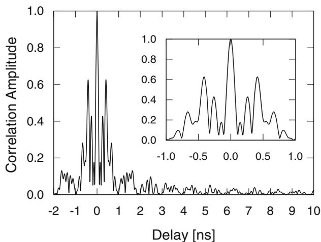
**Fig. 7** Delay-resolution function for the array of frequency bands centered on 6.0, 8.5, 10.4, and 13.3 GHz with 1024 MHz width each. This array was used for the intercontinental broadband VLBI between Medicina–Kashima–Koganei discussed in Sect. 3.2. The plot focuses on the positive side of the symmetric function to provide greater detail. The inset shows a magnification of the behavior near 0 delay
