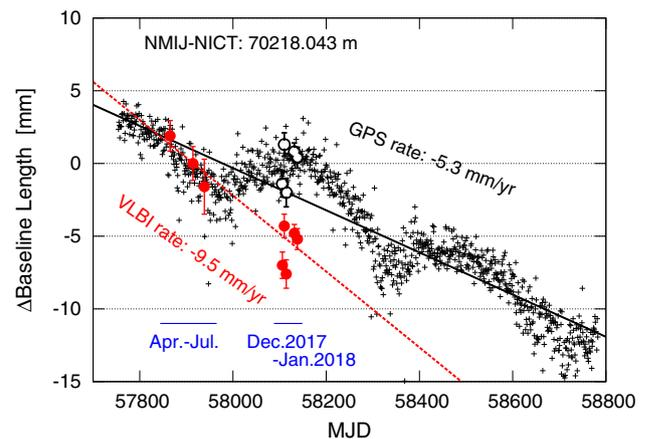
**Fig. 12** Time series of the baseline length measured by VLBI sessions in Table 3. Filled circles '●' indicate NHS VLBI results for the MARBLE1 - MARBLE2 baseline with error bars showing 1-sigma uncertainty of the solution. GPS-based baseline lengths are shown by '+' marks, vertically shifted to match the VLBI results. Open circles '○' represent a hypothetical shifted antenna position as given in the text
