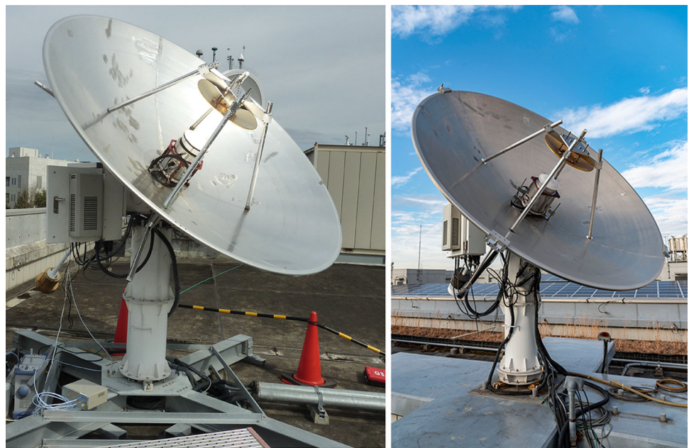
Fig. 10 (left) MBL1 at NMIJ (Tsukuba) free-standing on protective rubber pads, (right) MBL2 at NICT (Koganei). The temperature controlled 'receiver box' including filter, amplifier, and E/O device is visible behind the main reflector (see main text)
