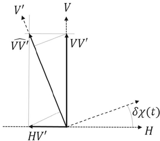
**Fig. 6** Emulated polarization-aligned cross-correlation data  $\widehat{VV'}$  are computed by linear combination of the cross-correlations for  $HV'$  and  $VV'$ , taking into account the parallactic angle difference  $\delta\chi(t)$
