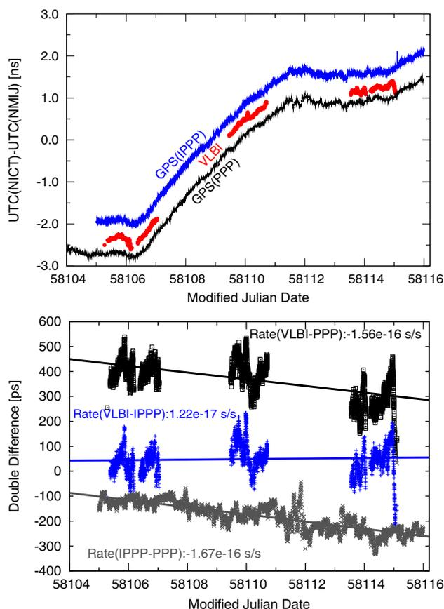
**Fig. 13** Time scale comparison of UTC(NICT)–UTC(NMIJ) with broadband VLBI, GPS(PPP), and GPS(IPPP). The lower panel shows the pair-wise double difference. Since a constant time offset is of no concern, data in both plots are offset for visibility
