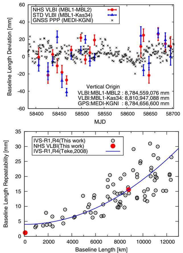
**Fig. 16** Upper panel shows baseline lengths (as deviation from the value specified in the figure) measured by VLBI and GPS PPP solutions of similarly located MEDI and KGNI stations. Lower panel shows BLR for MBL1–MBL2 (‘●’) and our re-evaluation of IVS-R1 and R4 sessions during 2011–2013 (‘○’). The solid line represents a regression function of BLR for IVS-R1 and R4 sessions in a preceding study (Teke et al. 2008)
