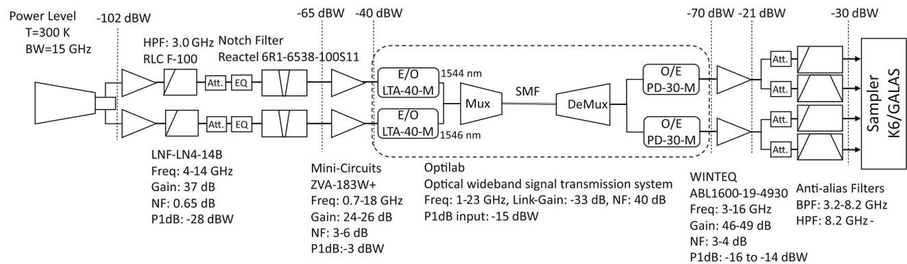
**Fig. 2** Block diagram of the receiving signal chain for the data acquisition of Kas34. Dual (V & H) linear polarization signals are transferred from the receiver room of the antenna to the observation room through one single mode fiber (SMF) using a wavelength division multiplexer (Mux) and demultiplexer (DeMux). For efficient data acquisition, equal-
