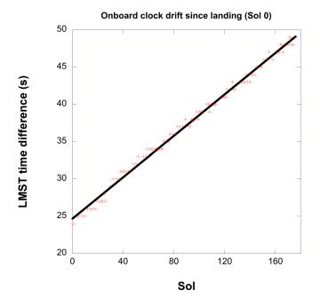
**Figure 4.** Drift in the Local Mean Solar Time due to the free-running onboard clock on InSight spacecraft. Here, the LMST time difference corresponds to the difference between the onboard time converted using WebGeocalc algorithm and Savoie et al. (2019) algorithm, expressed as integers. The data are plotted for 6 months from Sol 0 (November 26th, 2018). The dark line is fitted to the data, and corresponds to a linear increase of the drift of 0.139 s per sol.
