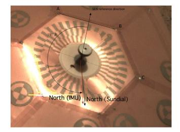
**Figure 8.** Comparison between sundial north determination and IMU north direction.
