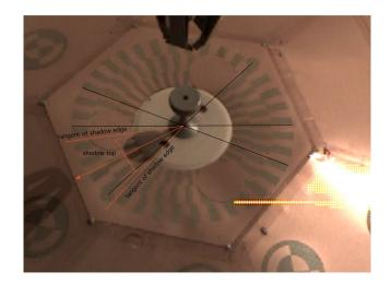
**Figure 5.** Estimation of the shadow direction on the image taken on 01/01/19 at 15 h 33 m 33 s LMST. Dark rays define the shadow center and red rays define the shadow border, shadow top tangent and shadow top direction.
