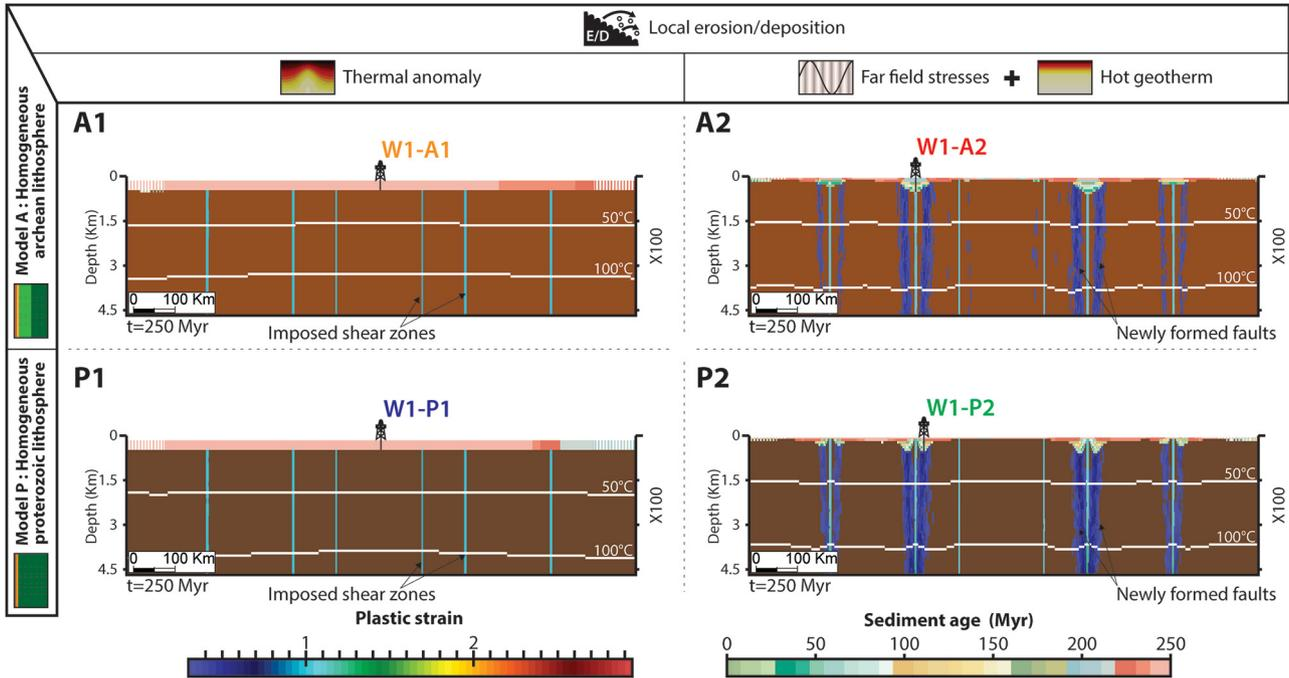
**Fig. 5.** (A1) Model A with thermal anomaly shows no creation of basin. (P1) Model P with thermal anomaly shows no creation of basin. (P2) Model P with far field stresses shows the creation of eight narrow basins with chaotic stratigraphic architecture near shear zones. (A2) Model A with far field stresses displays the formation of four narrow basins with chaotic stratigraphic architecture above shear zones.
