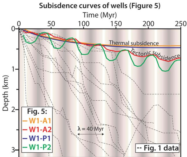
**Fig. 6.** Subsidence curves from different models in Figure 5 (wells W1-A1 to W1-A2 and W1-P1 to W1-P2) associated with Figure 1 bibliographic data (dashed lines). The thermal subsidence of W1-A1 and W1-A2 is achieved after 150 Myr. The wells P1 and P2 show linear decay subsidence with deviations of different amplitudes. See Figure 4B for the boundary conditions.
