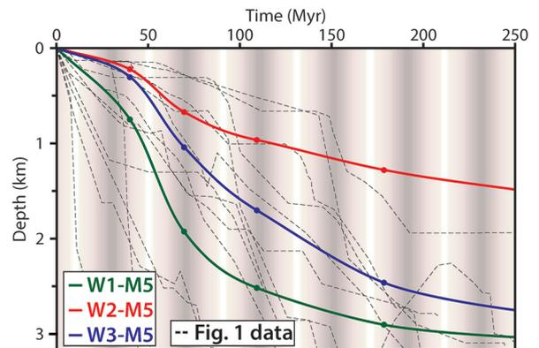
**Fig. 9.** (A) Tectono-stratigraphic basin architecture and heat production of Model M5 without thermal anomaly shows stratigraphic features (*i.e.* onlaps, truncations and thickness variations) when approaching the arches. (B) Stratigraphy and hiatus repartition between the wells W1-M5 to W3-M5. (C) Subsidence curves of well W1-M5 to W3-M5 are characterized by exponential decay shape. Comparison with [Figure 1](#) subsidence bibliographic data (dashed lines).
