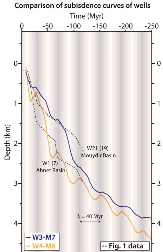
**Fig. 12.** Comparison of total subsidence curves between numerical models and geological data extracted from the Mouydir Basin, Algeria (9: Well W21; Perron *et al.*, 2018) and the Ahnet Basin, Algeria (5: well W1, Kracha, 2011). The Algerian wells are localized in Figure 2A. The curves are presented in Figure 1.
