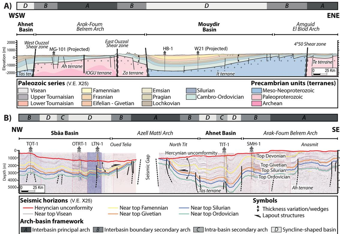
**Fig. 3.** (A) WSW-ENE geological cross section of the Mouydir Basin showing typical arch and basin architecture defined as a syncline-shaped basin with boundary secondary arches. (B) NW-SE seismic profiles of the Ahnet Basin defined as a complex shaped basin with intra-basin arches. The specific zonation of the terranes age with the arches-basins architecture is observed (see also Perron *et al.*, 2018).
