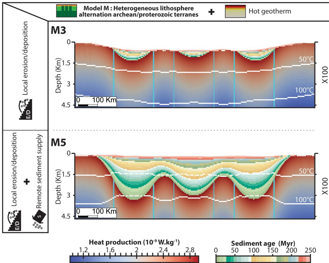
**Fig. 10.** Comparison between model M3 and M5 showing increase of basin depths and the deposits on the arches in case on higher sediment supply due to remote sediment supply. One may note also that the temperature in the basin and in the crust is affected by this higher sedimentation rate, it is due to heat production of the basement. The isotherms rise up below the basins and down below the arches.
