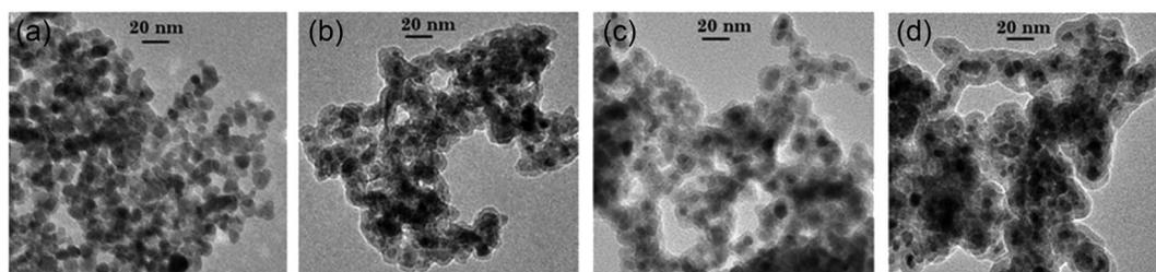
Fig. 4 TEM pictures of  $\text{ZnGa}_2\text{O}_4:\text{Cr}^{3+}, \text{Bi}^{3+}$  nanoparticles (a) after silica layer removal, (b) with a 3 nm silica layer, (c) with a 5 nm silica layer and (d) with a 10 nm silica layer.
