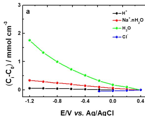
**Figure 7.** Evolution of the relative concentration,  $C_i - C_0$  of each species over the potential applied measured in 0.5 M NaCl SWCNT/PPy.
