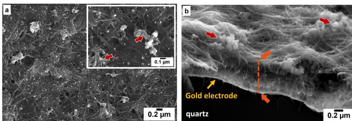
**Figure 1.** FEG-SEM images of single-wall carbon nanotubes/polypyrrole (SWCNT /PPy) nanocomposite film deposited on the gold electrode of a quartz resonator: (a) surface morphology with an inset showing the PPy clusters and (b) cross-section (red arrows point out the PPy clusters and orange colored arrows show the average film thickness).
