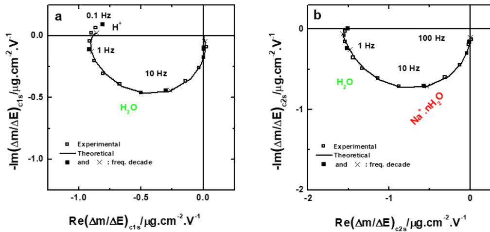
**Figure 5.** Partial electrogravimetric transfer function of the SWNT-PPy thin film in 0.5 M NaCl measured at  $-0.4$  V vs. Ag/AgCl: (a)  $\left. \frac{\Delta m}{\Delta E} \right|_{c1s}(\omega)$  cation1-solvent partial transfer function and (b)  $\left. \frac{\Delta m}{\Delta E} \right|_{c2s}(\omega)$  cation2-solvent partial transfer function. Theoretical functions were calculated with the same set of parameters used previously for the data presented in Figures 3 and 4.
