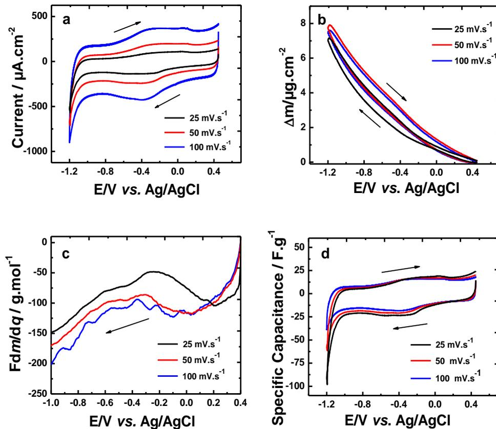
**Figure 2.** EQCM results of SWCNT/PPy composite thin films: (a) current vs. potential; (b) mass variation vs. potential; (c) calculated  $F \frac{dm}{dq}$  values vs. potential; (d) specific capacitance values (calculated from panel a) vs. potential. Measurements in aqueous electrolyte 0.5 M NaCl pH 7.0 at 3 different scan rates.
