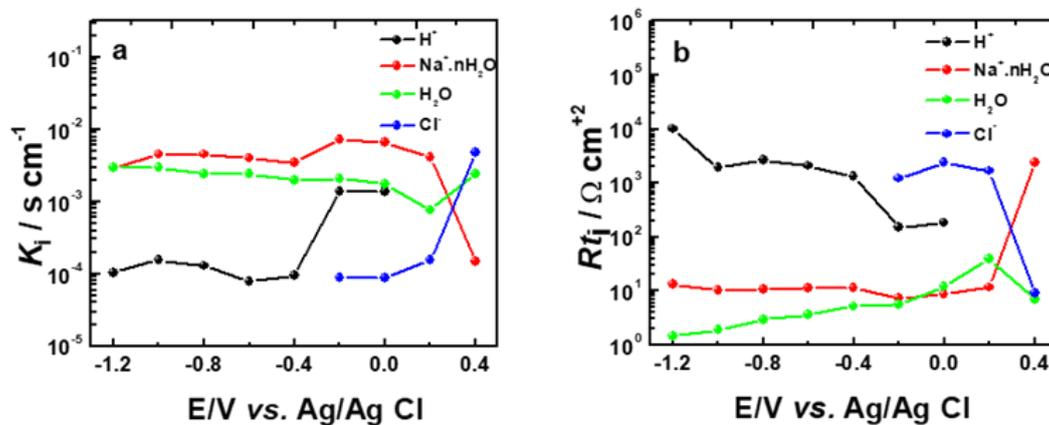
**Figure 6.** The kinetic transfer constants,  $K_i$ , and transfer resistance,  $R_{t_i}$ , for all species estimated from the fitting of the  $Ac$ -electrogravimetric data of SWCNT/PPy composite measured in 0.5 M NaCl: (a) kinetic transfer constants,  $K_i$  and (b) transfer resistance,  $R_{t_i}$ .
