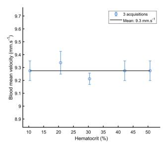
**Figure 3.** Measurement of mean blood velocity at a flow rate of 0.25 mL/min and for 5 hematocrit values. The measurement was performed from the blood volume ejected at the output of the experimental set-up during 4 min.
