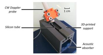
Figure 1. Picture of the probe and the tube mounted in the 3D-printed support.
