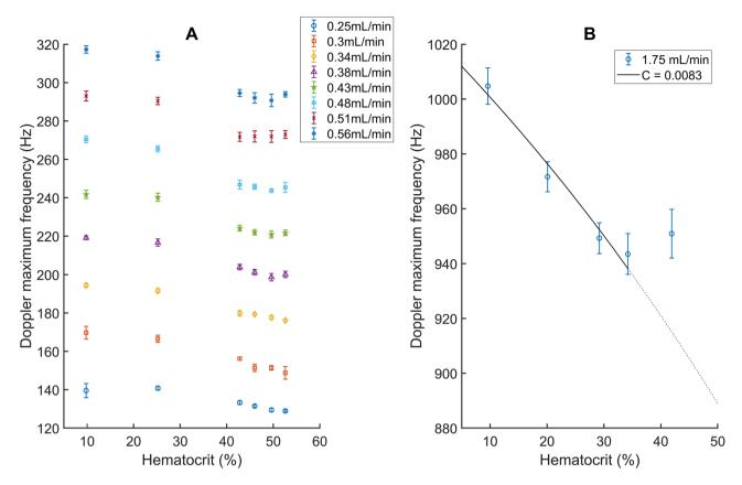
**Figure 2.** Experimental demonstration of the method flow rate dependency for the single tube radius used. The decrease of Doppler maximum frequencies saturates for an hematocrit superior to 50% if the flow rate is above or equal to 0.38 mL/min (**A**). The saturation effect has been observed for flow rates up to 1.75 mL/min (**B**). In (B) A fit of Eq. (7) has been performed but only for hematocrits where no saturation effect was observed.
