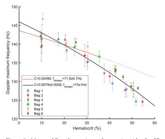
**Figure 5.** Measured Doppler maximum frequencies with a fit of Eq. (7) (black line) and with a fit of Eq. (7) restricted to hematocrits under 35% (red line). The fit on the whole hematocrit range has been performed with C and  $f_{dmean}$  as fitting parameters and the restricted fit has been performed with  $f_{dmean}$  as the only fitting parameter and with C fixed to the Walburn and Schneck value (1976).
