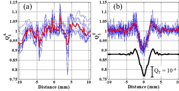
Figure 3 : Detection of ratio  $Q_I^A$  (a) and  $Q_I^T$  (b) from single shot detection (dot blue lines) and averaging of 10 detections (red continuous line). On (b), the signal presented in black (with its own amplitude scale) is obtained from linear simulations of a static inclusion.
