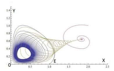
FIGURE 8. Plot of an orbit of the non-autonomous system (11), (12), starting from the vicinity of E. Initially it is somewhat analogous to the solution for the autonomous system with the initial values of the parameters, but afterwards it evolves approaching gradually of the asymptotic limit, corresponding to the final values of the parameters. Two orbits for the autonomous systems corresponding to the initial and final values of the parameters are also plotted.
