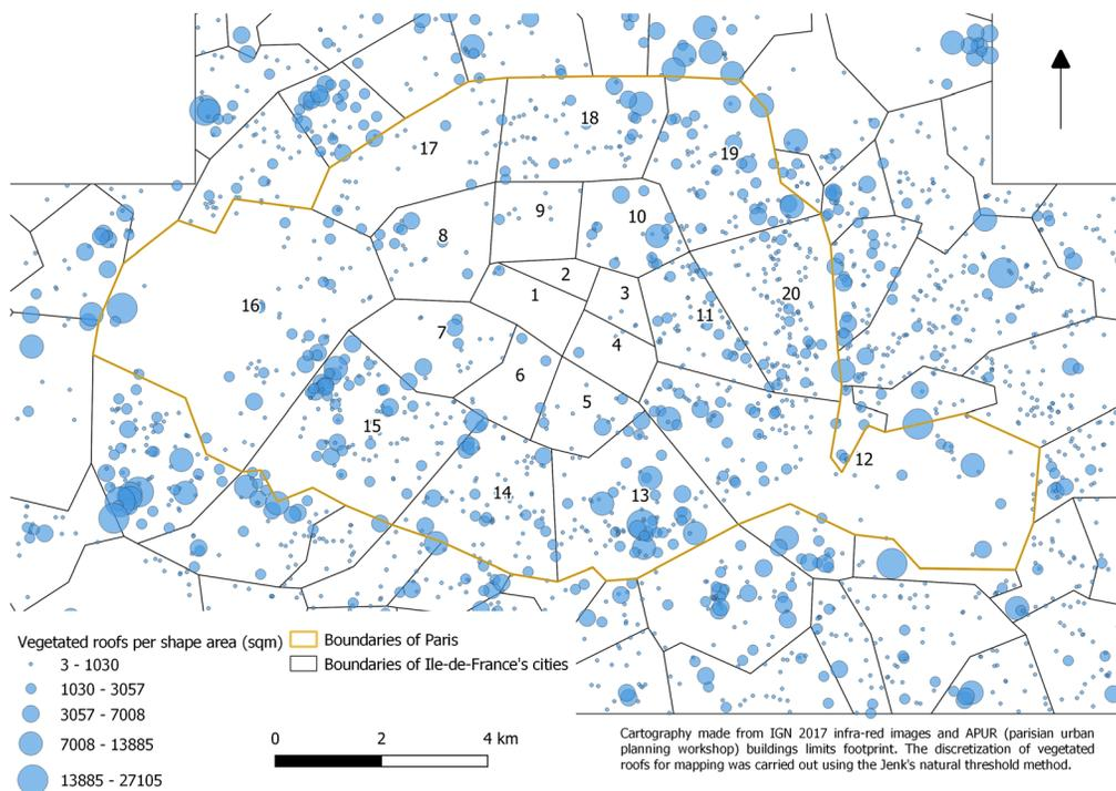
**Fig. 7** Vegetated roofs resulting from our modeling, depending on building shape area, centered on Paris.
