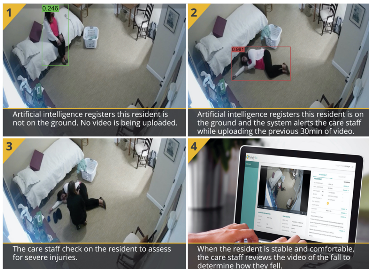
Figure 1. SafelyYou Guardian (SYG) technology provides automated notification of the fall, video footage (to assess fall severity), and care recommendations to facility staff.
