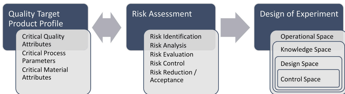
Fig. 2. The schematic flow-chart of Quality-by-Design ideology. First, critical quality attributes, critical process parameters, and critical material attributes must be defined, and their relationships clarified. Second, risk assessment is performed. Third, design of experiment is conducted by scientifically determining the relationships between process factors. Risk assessment and quality target product profile are constantly reflected to each other to optimize the outcome.
