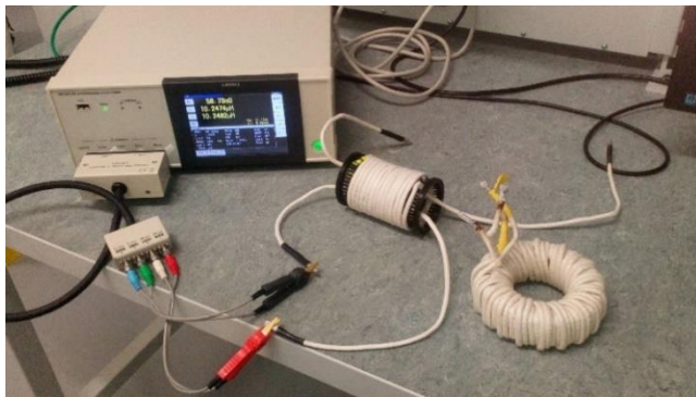
Fig. 3: test bench for air core transformer
