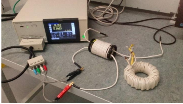
Fig. 3: test bench for air core transformer
