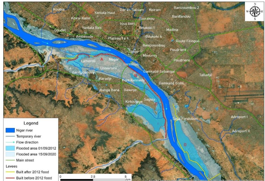
**Figure 19.** Comparison of Niamey flooded areas in 2012 and 2020 events. The red letters identify the four levee sectors: (A) Lamordé, (B) bridges, (C) Kirkissoye-Saguia and (D) Saga.
