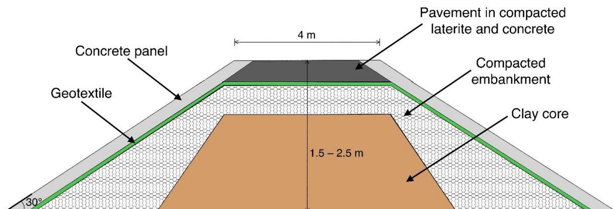
**Figure 6.** The cross-section of Niamey levees in the Lamordé (sector A) and Saga (sector D).
