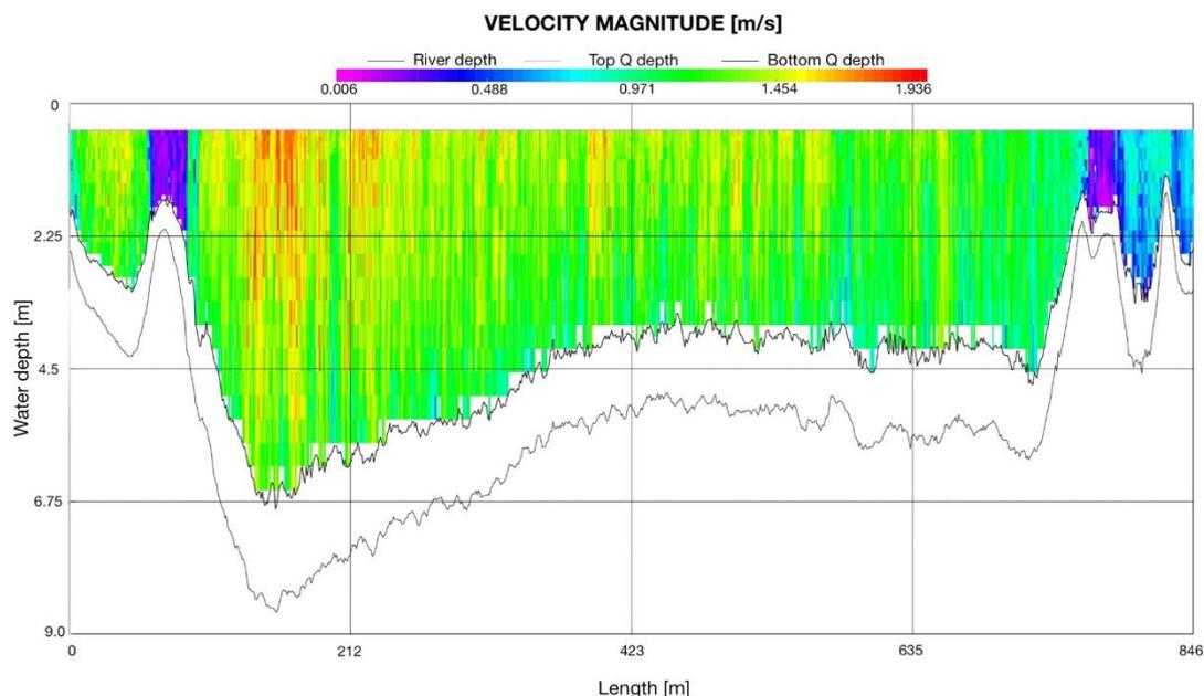
**Figure 3.** Acoustic Doppler Current Profiler (ADCP) observation conducted in the Niger River in Niamey (Soumana section) on 8 September 2020 with a flow depth of 698 cm (2850 m<sup>3</sup>/s).
