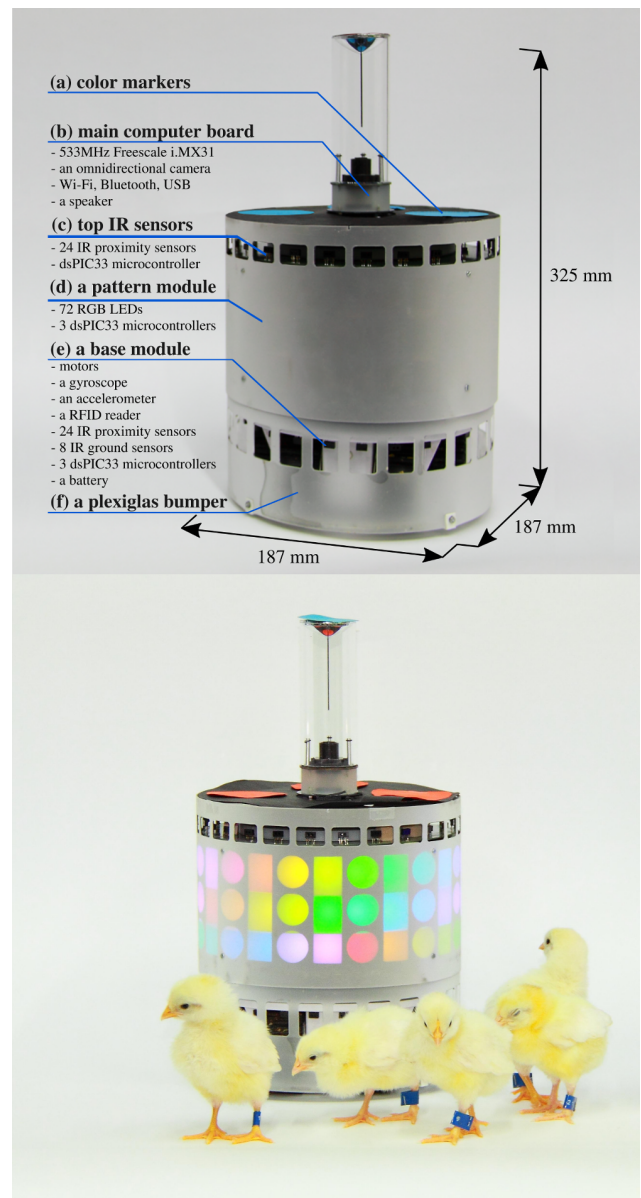
FIG. 1: The PoulBot autonomous robot. The robot developed to test individual and social behaviour among chicks is based on the modular research robot marXbot 13 . This robot is equipped with a plastic shell that prevent chicks from being roll over or stuck in the tracks. The upper side of the shell allows to display a predefined colour pattern. The tube on the top is a 360° omnidirectional camera that allows the robot to perceive visually its surrounding. The small rectangular holes allow infra-red sensors to detect objects or animals in close vicinity.
