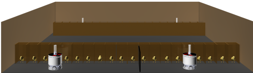
FIG. 17: Design of the imprinting set-up. The robots travel back and forth between two walls in front of the chicks.
