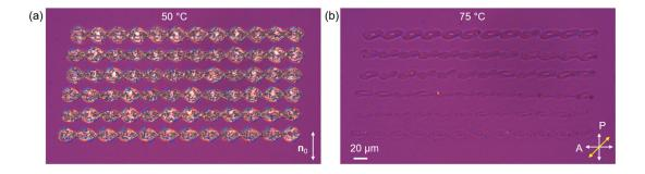
**Fig. 7** Surface-attached LCE microstructures. A lattice made of elastomeric microrings is constructed on the surface of a glass substrate. The sample (a) is heated above the phase transition temperature (b) of the polymerized LCE such that actuation of individual particles and changes of topology are observed.
