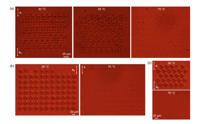
**Fig. 6** Elastomeric colloidal crystal lattices in a LC host. Micrographs are taken under different temperatures for originally close-packed hexagonal (a), sparse-packed square (b), and sparse-packed hexagonal (c) lattices. The repeating units are the microrings suspended in the LC host and not connected to each other, so that the particles are free to move around.
