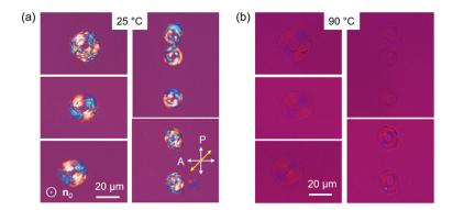
**Fig. 5** Surface-adhered LCE microrings made in homeotropic LC cells. In contrast to the ones in Fig. 4, shape change of these microrings is axially symmetric and isotropic in the viewing plane, though change of topology from genus-zero to genus-one is also observed, as shown in the bottom left corner. Far-field director  $\mathbf{n}_0$  during printing is perpendicular to the viewing plane as indicated by the circled dot symbol.
