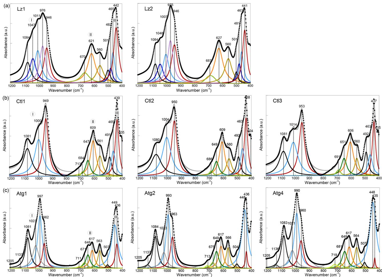
**Figure A1.** MIR spectra in the  $1200\text{--}400\text{ cm}^{-1}$  range (lattice transitions) of (a) lizardite (Lz1, Lz2), (b) chrysotile (Ctl1, Ctl2, Ctl3), and (c) antigorite (Atg1, Atg2, Atg4). The spectra have been decomposed into individual components using Lorentzian functions. Black dots: experimental data. Solid grey line: best fit. (I) Si–O stretching vibrations, (II) libration and hindered translation of OH groups, and (III) Si–O bending vibrations.
