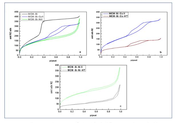
Figure 6. Nitrogen adsorption isotherms at -196 °C (77 K) for the different prepared materials. (a) MCM–Si and MCM–Si–M materials (M = Cu II, Ni II); (b) MCM–Si–Cu and MCM–Si–Cu–HT materials; (c) MCM–Si–Ni and MCM–Si–Ni–HT materials.
