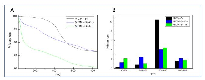
**Figure 3.** Thermogravimetric analysis (TGA) of MCM–Si and MCM–Si–M materials (M = Cu II, Ni II) plotted as a function of temperature versus % mass loss. Graphic representation with total analysis (**A**). Bar graph of temperature groups to illustrate mass loss trends (**B**).
