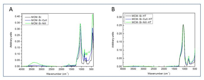
Figure 2. FTIR spectra of MCM-Si-M materials (M = Cu II, Ni II). Before (A) and after thermal treatment (B).
