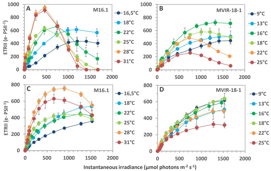
**Figure S1:** Photosystem II electron transport versus irradiance (photosynthesis / Energy; P/E) curves recorded by pulse amplitude modulation fluorometry. The initial slope  $\alpha$  and the saturation irradiance  $E_K$  were retrieved by fitting the Platt model (7). Curves recorded at 540 nm for *Synechococcus* spp. M16.1 (A) and MVIR-18-1 (B) at different growth temperatures. Curves recorded at 480 nm for *Synechococcus* spp. M16.1 (C) and MVIR-18-1 (D) at different growth temperatures.
