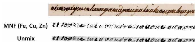
Fig. 8. Recovering the text using unmixing procedure. Details of page 1 of document 440AP_1_1_8, written by AF, 8 October 1791. Comparison of MNF maps and unmixing procedure. Read text: “et Sophie m’en voudra j’avoue qu’après.”
