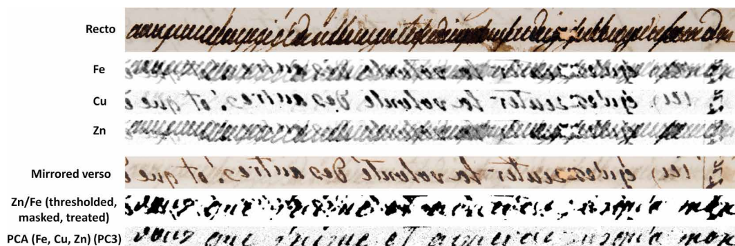
Fig. 4. Recovering the text using PCA. Details of page 5 of letter 440AP_1_1_2, written by MA, 7 December 1791. Elemental maps, mirrored verso, elemental ratio maps, and PCA of these details (4.8 mm by 116.1 mm; 100 \mu\text{m} ; 500 ms per pixel). Read text: “vous que j’aime et aimerai jusqu’a mon.”
