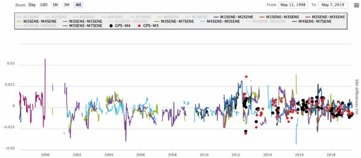
Figure 8. Time series of the SSH differences between Senetosa tide gauges (MiSENE where i is the tide gauge number and SENE is the abbreviation of Senetosa). The black dots and red diamonds correspond to the SSH differences with our GNSS-based sea level measurement system.
