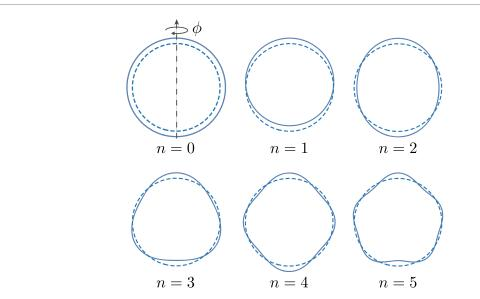
**Figure G1.** Schematic illustration of the lowest-order, axisymmetric, perturbative modes. The modes n=0 to n=5 are represented with an arbitrary amplitude. In each schematic representation, the unperturbed spherical shape is represented with a dashed line. In the first, n=0 mode, the axisymmetry is indicated as a rotational invariance in  $\phi$ , and all modes depicted here are invariant under this transformation.
