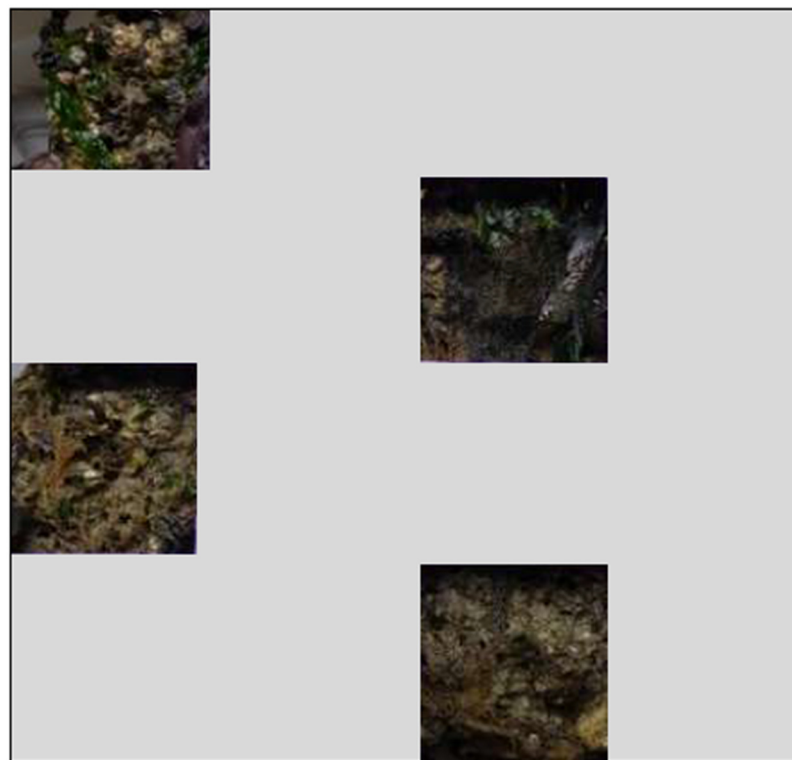
Figure 3. Photo of a block showing a mask of 5 \times 5 \text{ cm} , i.e., 25 \text{ cm}^2 .
