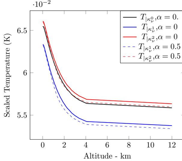
FIG. 5. Temperatures in Kelvin divided by 4,798 versus altitude, computed with  $\kappa_\nu^0$ ,  $\kappa_\nu^1$ , and  $\kappa_\nu^2$  without scattering ( $\alpha = 0$ ) and with a scattering  $\alpha = \frac{1}{2}$ .
