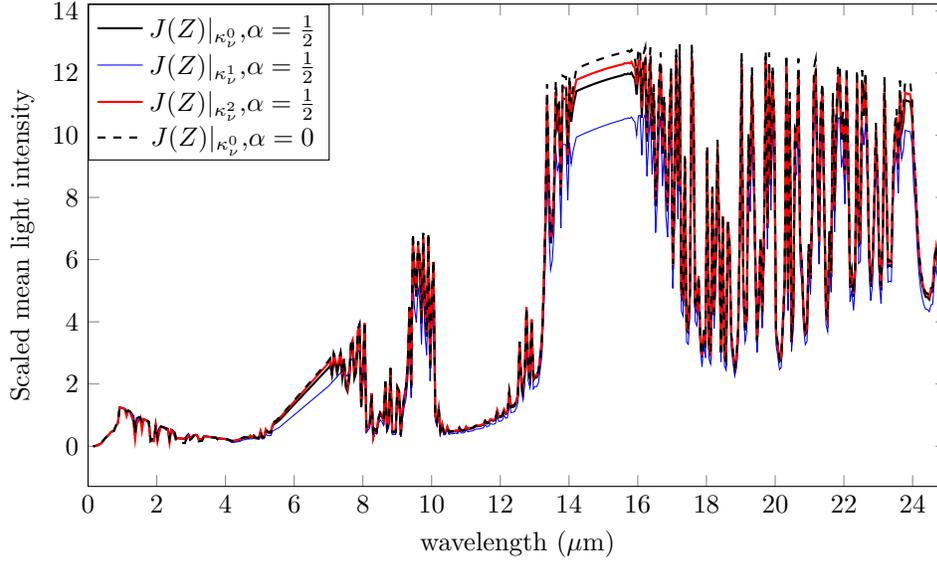
FIG. 4. Computed mean radiation intensities  $10^5 \cdot J_\nu(Z)$  at the top of the troposphere for  $\kappa_\nu^0$ ,  $\kappa_\nu^1$ ,  $\kappa_\nu^2$  with scattering ( $\alpha = \frac{1}{2}$ ) and for  $\kappa_\nu^0$  without scattering.
