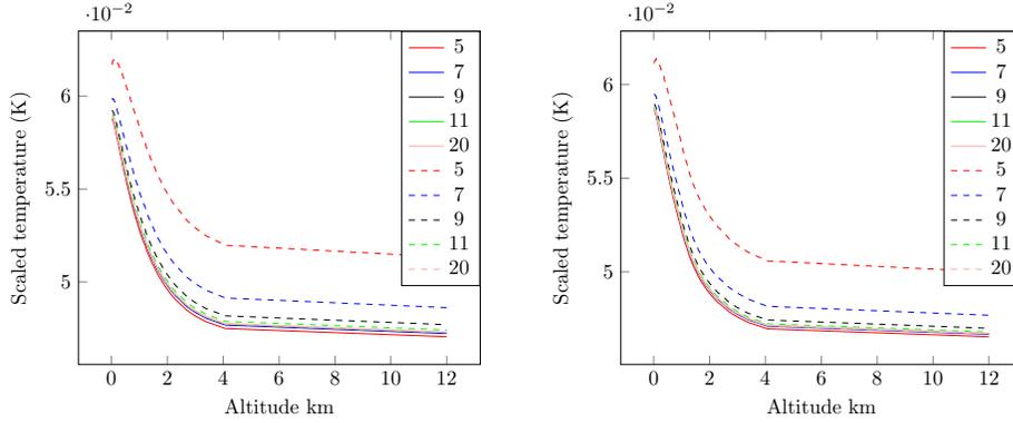
FIG. 2. Temperatures scaled by 4,798 without (left) and with (right) scattering: convergence history. The dashed curves are computed with an initial  $T^0 = T_{Sun}/10$  and the solid curves with  $T^0 = 0$ . Notice the monotonic convergence towards a solution after 20 iterations. The iterations shown for the upper and lower solutions are (5, 7, 9, 11, 20). This computation has used  $Q_0 = 3 \cdot 10^{-5}$ .
