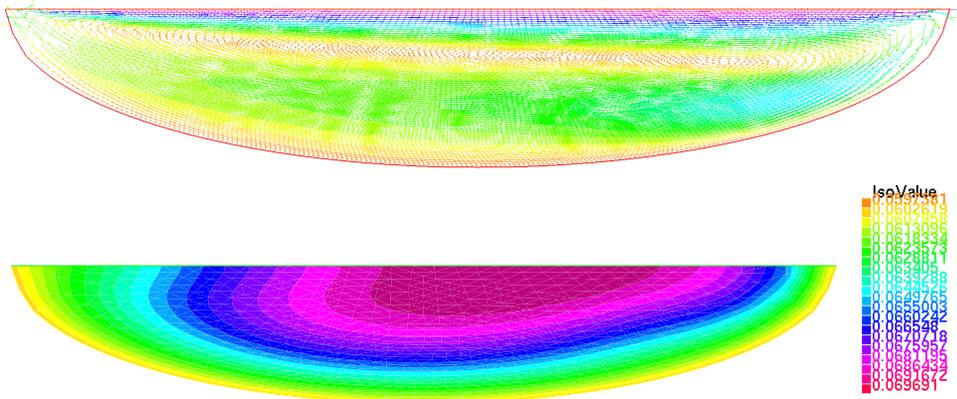
FIG. 6. *Velocity vectors and temperature in a pool subject to wind on its top boundary and given temperature on the bottom. The wind creates a large eddy rotating clockwise which, in turn, moves the hotter fluid region to the right.*
