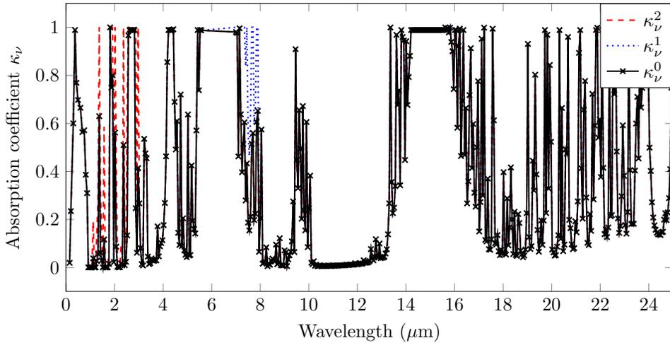
FIG. 1. Absorption  $\kappa_\nu^0$  versus wavelength ( $3/\nu$ ) read from Gemini measurements;  $\kappa_\nu^1$  is  $\kappa_\nu^0$  increased in the infrared range  $2-3\mu\text{m}$  and  $\kappa_\nu^2$  is  $\kappa_\nu^0$  increased in the range  $8-14\mu\text{m}$ . The  $\times$  marks show the 487 grid points for the integrals in  $\nu$ .
