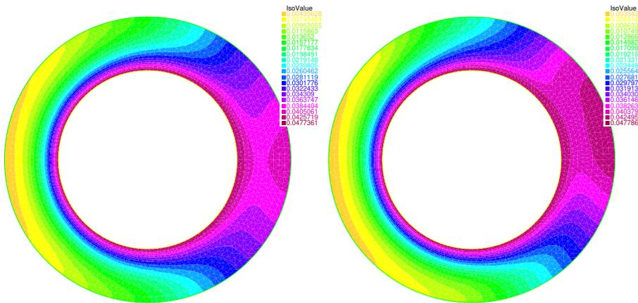
FIG. 8. *Temperature in the atmosphere of a planet heated by a sun on the right with wind (right) and without wind (left); it is a counterclockwise rotating wind around an axis almost (but not quite) perpendicular to the figure. Thermal diffusion propagates heat in unlit regions and the wind transports the heat counterclockwise. Note that the thickness of the atmosphere has been expanded for readability.*
