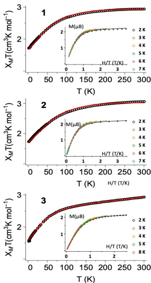
**Fig. 5.** Experimental and fitted simulated  $\chi_M T$  product against the temperature for 1-3. The inserts show the reduced magnetization plots for each compound at the quoted temperatures.
