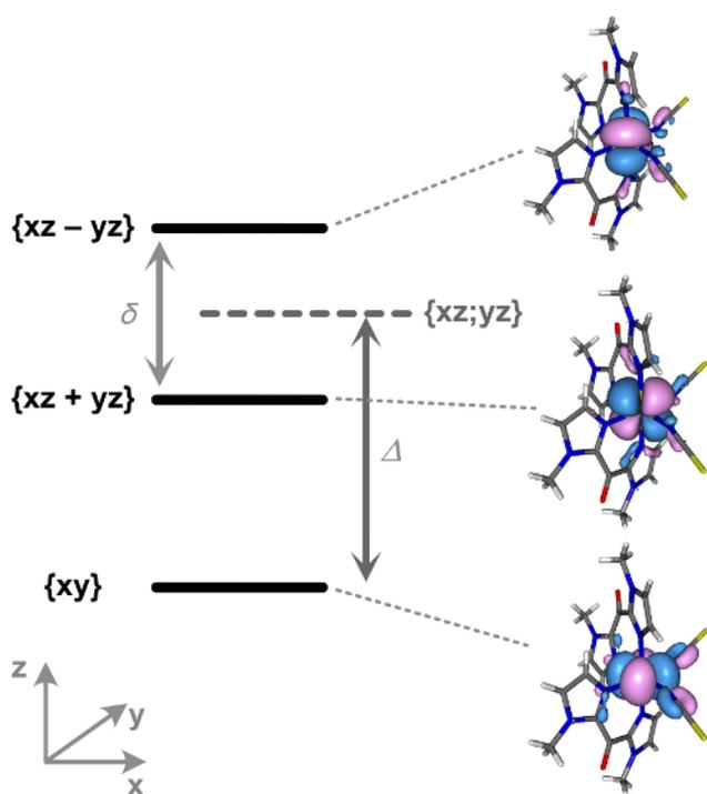
**Fig 3.** Splitting of the term energies obtained from a CASSCF/NEVPT2 calculation on the experimental geometries of **1** and **2**. The notation of the three states coming from the  ${}^4T_{1g}$  term in  $O_h$  symmetry was done with the only half-filled  $T_{1g}$  orbital.
