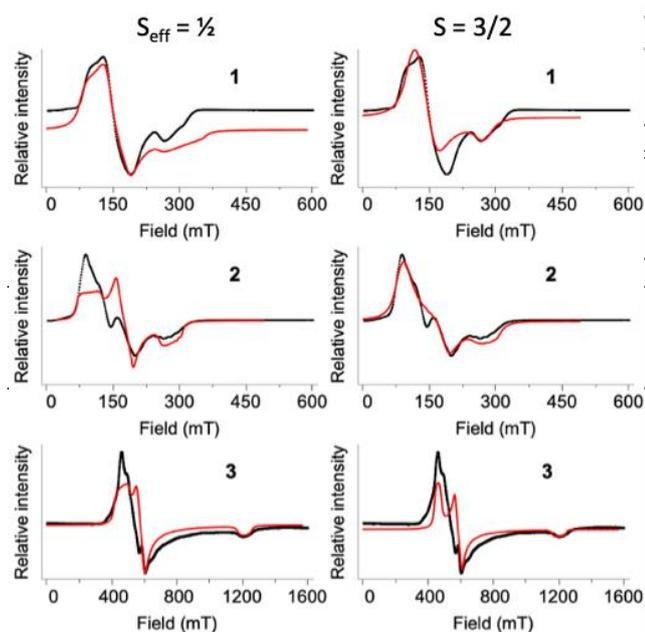
**Fig. 4.** Experimental (black) and simulated (red) powder X-band EPR spectra for 1-2 and powder Q-band for 3 at 4.0 K. The simulations have been carried out using an effective spin  $S_{\text{eff}} = 1/2$  (left column) and an anisotropic spin  $S = 3/2$  with  $E/D$  ratio obtained from *ab-initio* calculations (right column).
