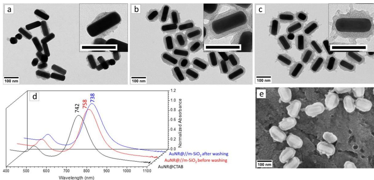
Figure 1. Results for protocol A, AuNR@m-SiO<sub>2</sub>: (a–c) TEM images taken at different reaction times: 5, 13, and 17 days, respectively. Scale bar in the inset corresponds to 100 nm. (d) Extinction spectra of the original AuNRs and AuNR@m-SiO<sub>2</sub> before and after washing for 17 days reaction time. (e) SEM images for (c).
