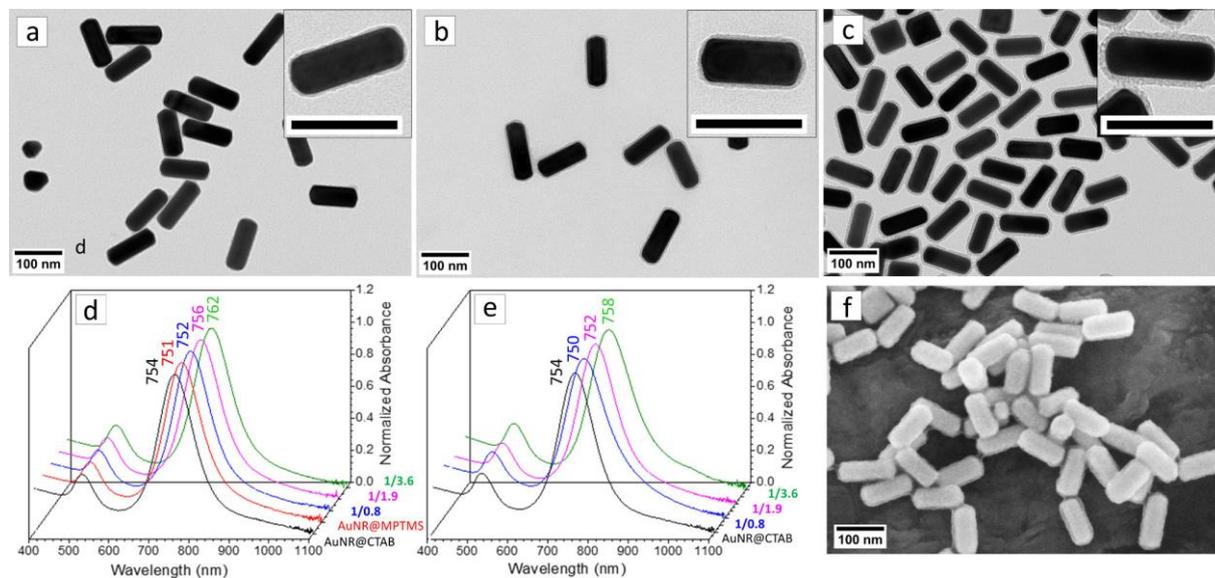
Figure 3. TEM images of AuNR@t-SiO<sub>2</sub> synthesized using MPTMS primer and pH monitoring with different Au/TEOS ratios: (a) 1/0.9, (b) 1/1.8, and (c) 1/3.6. Scale bars in the inset correspond to 100 nm. Extinction spectra of the obtained AuNR@t-SiO<sub>2</sub> (d) before purification and (e) after purification. (f) SEM image for (c).
