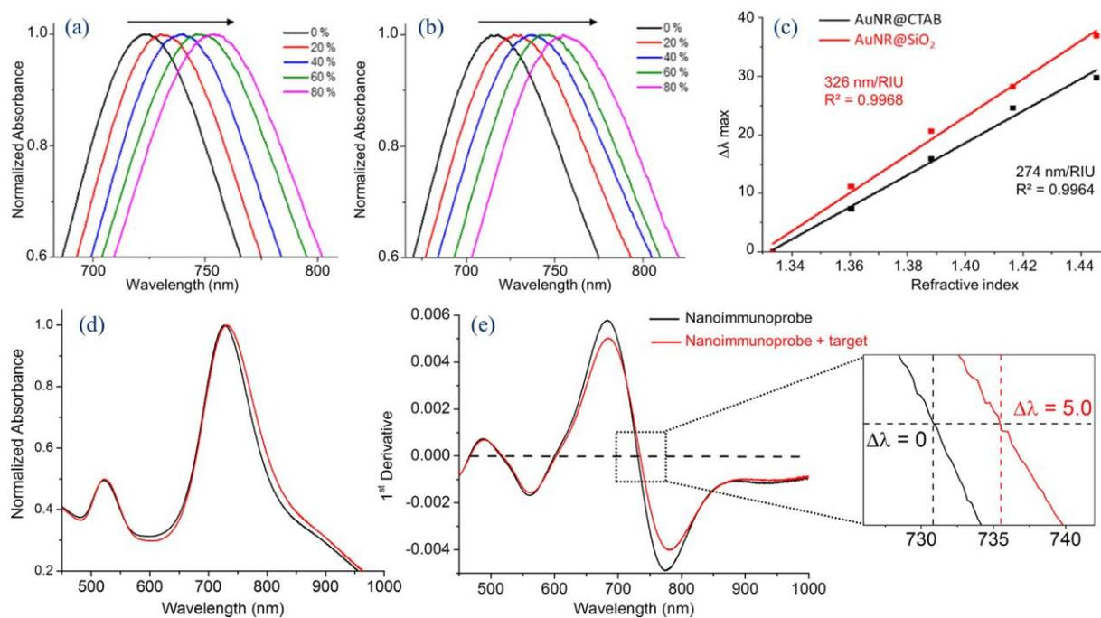
Figure 5. Normalized extinction spectra of (a) CTAB-capped AuNR and (b) AuNR@t-SiO<sub>2</sub> in water-glycerol mixtures of varying fractions; (c) dependence of the longitudinal plasmon shift of CTAB-capped AuNR (black squares) and AuNR@t-SiO<sub>2</sub> (red squares) on the refractive index of liquid mixtures. (d) Normalized extinction spectra of the nanoimmunoprobes before and after target recognition and their derivatives (e).
