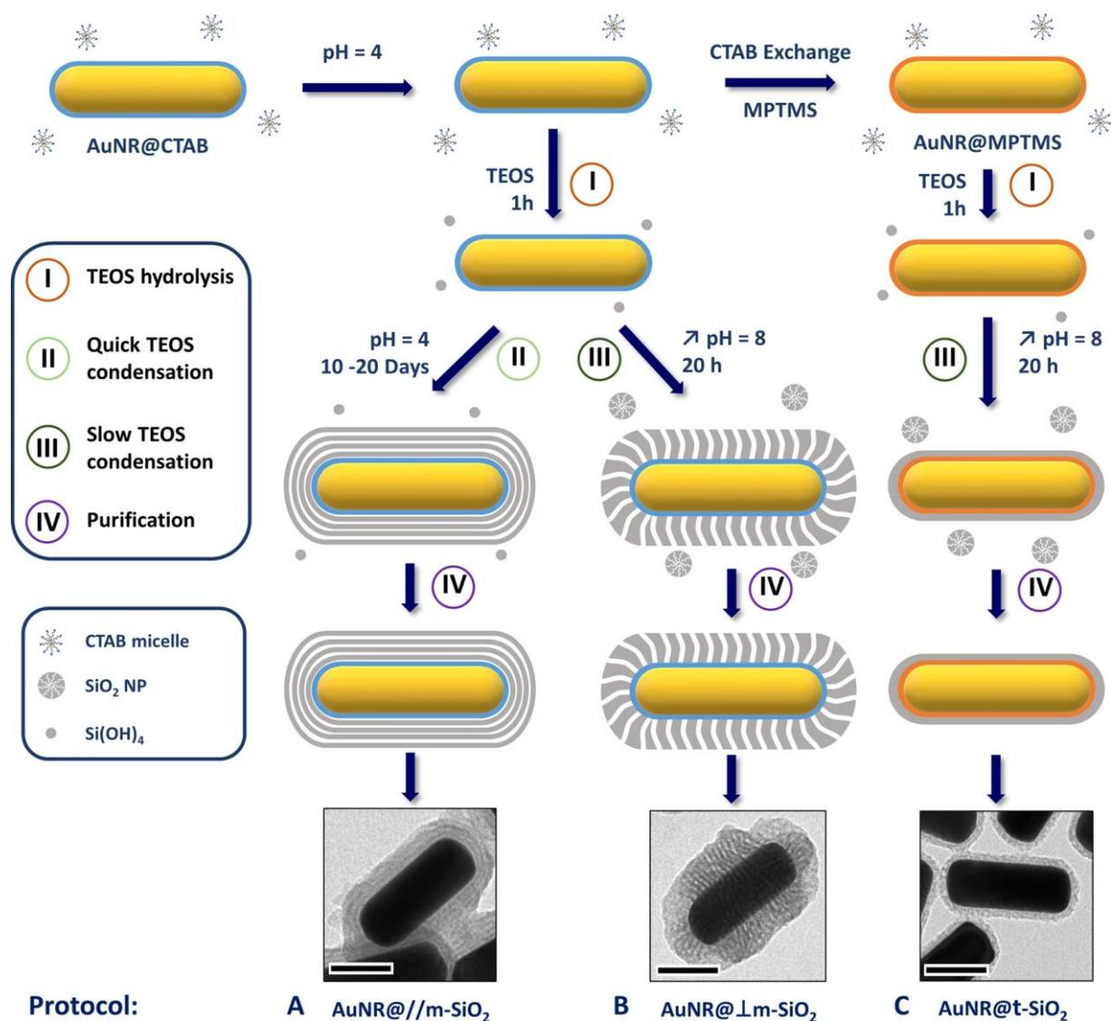
Scheme 1. Pathways Adopted for the Three Protocols Developed to Grow a Silica Shell on AuNRs: (A) AuNR@m-SiO<sub>2</sub>, (B) AuNR@l-m-SiO<sub>2</sub>, and (C) AuNR@t-SiO<sub>2</sub>
