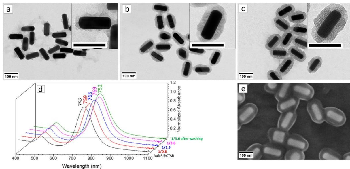
Figure 2. Results for protocol B, TEM images of AuNR@1m-SiO<sub>2</sub> synthesized with controlled NaOH addition and [CTAB] of 1.6 mM using different Au/TEOS ratios: (a) 1/0.9, (b) 1/1.8, and (c) 1/3.6. Scale bars in the inset correspond to 100 nm. (d) Extinction spectra of the original AuNRs and AuNR@1m-SiO<sub>2</sub> using different Au/TEOS ratios before and after washing. (e) SEM image for (c).
