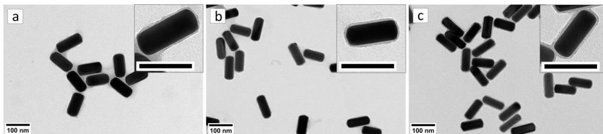
Figure 4. TEM images of AuNR@t-SiO<sub>2</sub> synthesized using the MPTMS primer and pH monitoring at a 1/1.8 Au/TEOS ratio with different AuNR dimensions: (a) 109 × 49 nm<sup>2</sup>, (b) 94 × 39 nm<sup>2</sup>, and (c) 102 × 36 nm<sup>2</sup>.
