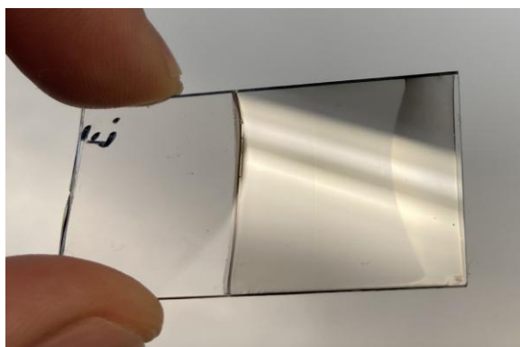
Figure 5 Photograph of the dip-coated mesoporous Ru-based film obtained at 300°C
