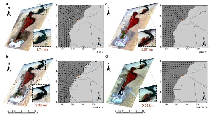
**Fig. 3.** Exemplification of two time intervals in which there was a wide opening of the inlet (**a** and **b**, 12 November 1990 and 08 September 2007, respectively) and the other two where there was a partial closure (**c** and **d**, 26 December 2006 and 06 January 2011, respectively) through satellite image and wind data at sea level. The red dot represents the studied area of approximated localization. NOAA/NCDC blended daily global 0.25° sea surface winds. Data courtesy of NOAA NCEI.
