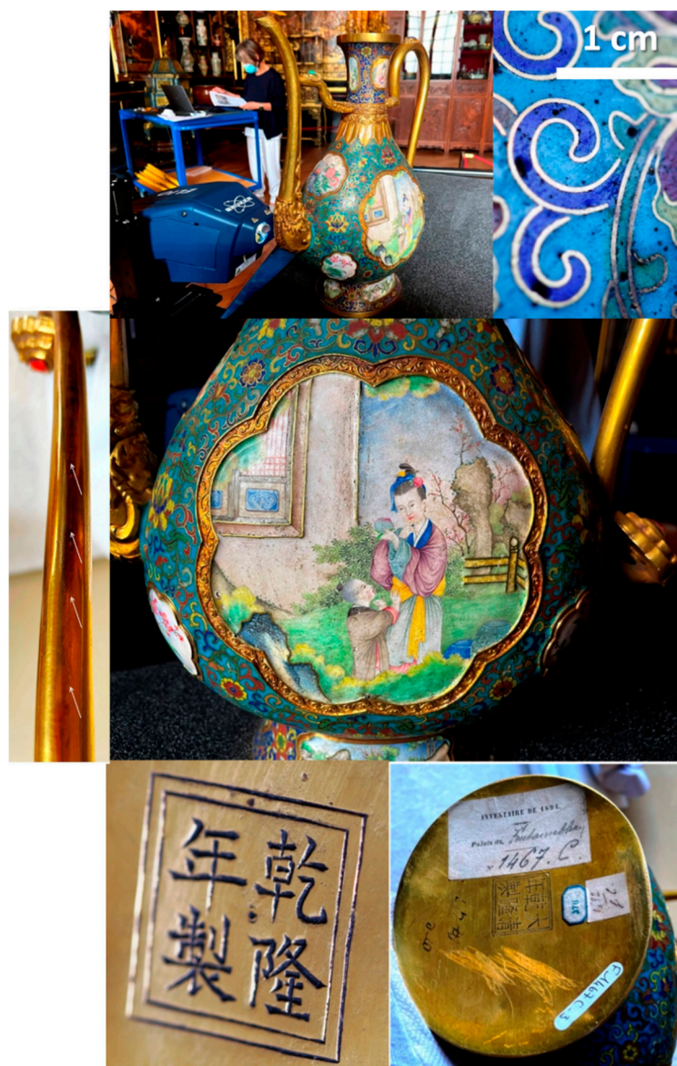
Figure 1. On-site pXRF analysis of the enameled ewer (F1467C) and details of the décor ( cloisonné and painted enamels); the bottom face exhibits an engraved Qianlong reign mark (bottom left, basin: Qian long nian zhi ; right, ewer; Da qing Qian long nian zhi ). Note the welding traces along the spout (arrows).
