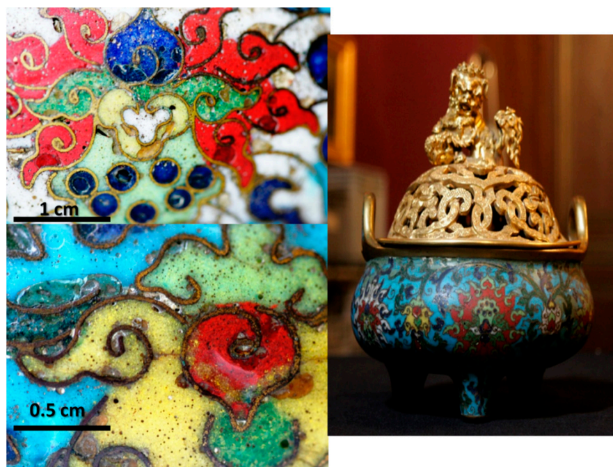
Figure 2. The incense burner (F1448C) and details of the cloisonné enameled décor (Kangxi reign). Note the many bubbles in the décor revealed by surface polishing.
