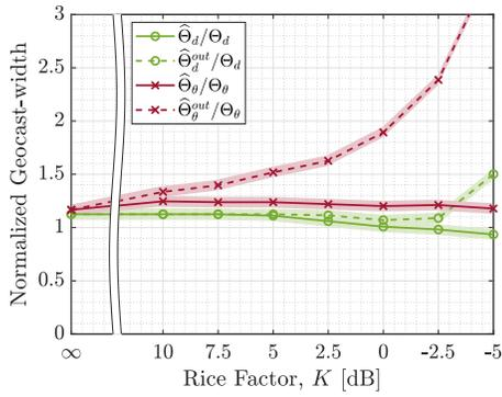
Fig. 7. Geocast-width and outlier-inclusive geocast-width (normalized) for decreasing Rice factor  $K$ . Shading shows uncertainty ( $\pm 2\Delta d_{sim}$ ,  $\pm 2\Delta\theta_{sim}$ ) due to discretized simulation grid.
