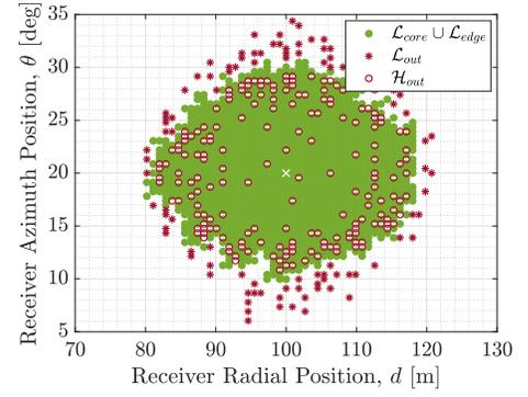
Fig. 9. Clustering results for OFDM-SDF geocast delivery zone identification at Rice factor  $K = 2.5$  dB and target position ( $d^{steer} = 100$  m,  $\theta^{steer} = 20^\circ$ ), marked by white  $\times$ .
