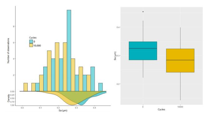
**Figure 4.** Histogram, density and boxplot of the arithmetic mean deviation Sa computed for all the measurements closest to the edge, after using a high-pass filter with a cut-off length of  $25 \mu m$ .
