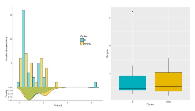
**Figure 2.** Histogram, density and boxplot of the arithmetic mean deviation (Sa) before (0 cycle) and after use (10,000 cycles). Sa values are computed for all the measurements closest to the edge, at full scale.
