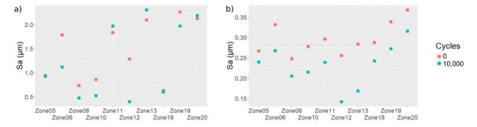
**Figure 5.** Arithmetic mean deviation (Sa) computed for the 10 selected measurements showing the largest wear traces (a) without filtering, (b) with filtering (high-pass filter with a 25 µm cut-off length).
