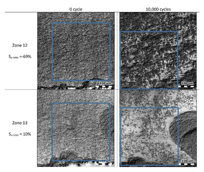
**Figure 1.** Photo simulation images of two locations and corresponding Sa ratios. Matching sub-surfaces are shown by the blue rectangles for each zone.
