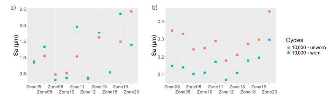
Figure 7. Arithmetic mean deviation (Sa) computed for the 10 selected measurements showing the largest wear traces. The Sa values are computed following the proposed methodology using masks (a) without filtering and (b) with filtering (high-pass filter with a 25  $\mu$ m cut-off length).
