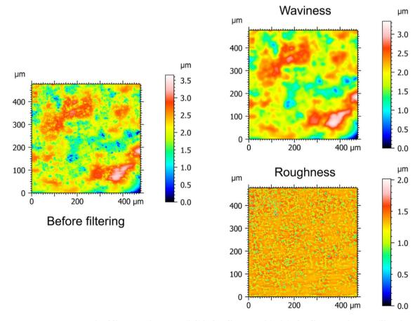
Figure 3. Example of filtering with Zone 12 (left) before filtering and (right) after filtering with a cut-off length of 25  $\mu$ m: as a high-pass filter is used, only the roughness part is kept for the analysis.
