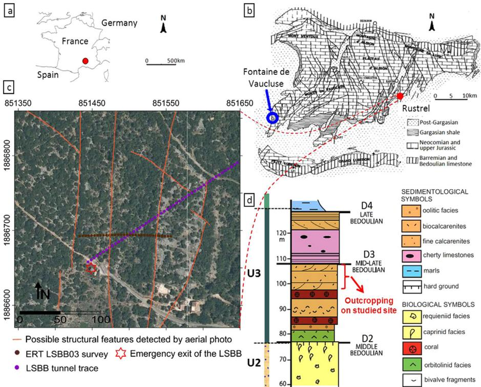
**Fig. 1.** (a) Fontaine-de-Vaucluse basin located in France; (b) Test site located in Fontaine-de-Vaucluse basin [4]; (c) Aerial photo with main lineament detection and survey location ([www.geoportail.gouv.fr](http://www.geoportail.gouv.fr)); (d) Regional lithostratigraphic log ([5] modified).
