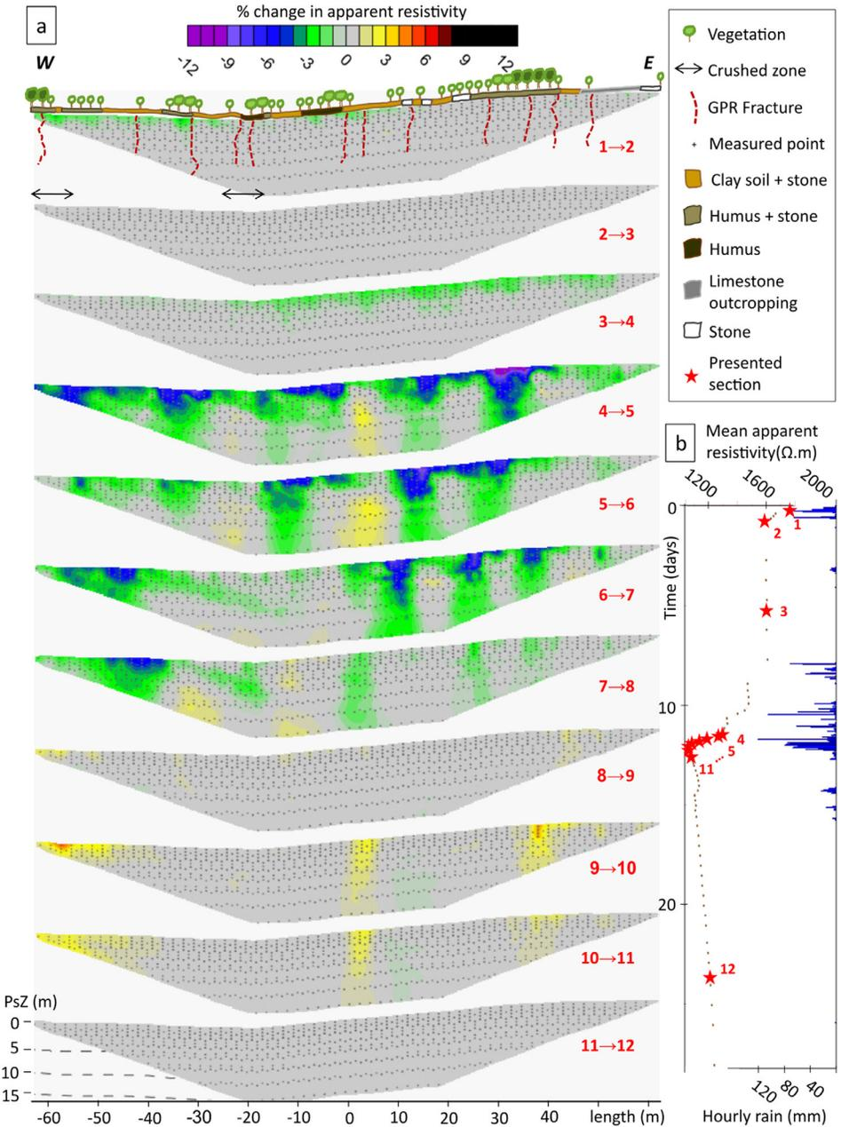
**Fig. 3.** (a) Hourly change in apparent resistivity between two consecutive time steps. Positioning of fracture detected by GPR and basic representation of vegetation and soil cover; (b) Evolution of mean apparent resistivity during monitoring versus rain [7]. Each brown point represents one ERT section.
