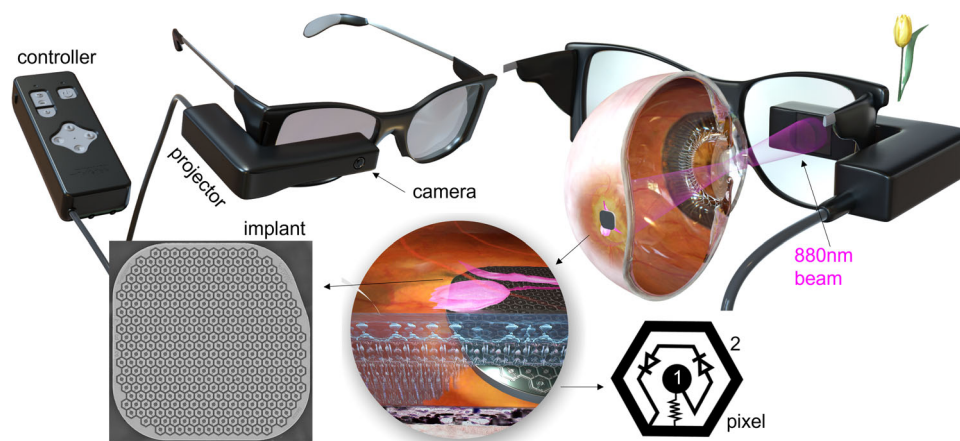
Fig. 1 Diagram of the PRIMA system. Top row: Artistic rendering of the augmented reality glasses with a projector and a camera. The 880 nm beam projects the video stream onto the retina. Bottom row: PRIMA implant with a hexagonal array of 100 \mu\text{m} pixels. Implant is placed under the degenerate retina without damaging the peripheral healthy retina. Pixels are composed of two photodiodes connected in series between the active (1) and a circumferential return (2) electrode.
