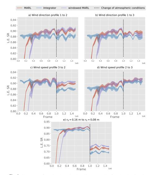
**Fig. 6.** Comparison of L.E. SR obtained in the evaluation episodes for MARL/windowed MARL and integrator controllers for experiments regarding changing atmospheric conditions.
