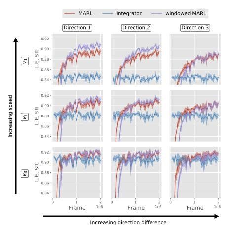
Fig. 5. Comparison of L.E. SR obtained in the evaluation episodes for MARL/windowed MARL and integrator controllers with different initial atmospheric conditions. Initially, the MARL controller has worse performance than the integrator controller, but after sufficient training, it surpasses the integrator controller in all cases.
