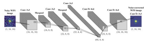
**Fig. 2.** Autoencoder for denoising WFS images. The tuple indicates the shape of the output at each step.
