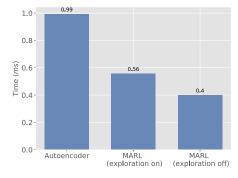
**Fig. 13.** Average inference time of all the components of the MARL controller for 1000 inferences in the closed-loop setting.
