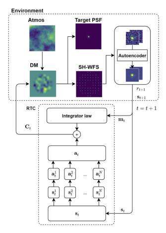
Fig. 4. Multi-Agent Reinforcement Learning for Adaptive Optics control. The environment, as seen from the Multi-Agent RL controller, is composed of the atmosphere, the DM, the WFS and the autoencoder that denoises the WFS image. The Multi-Agent RL will take the state as an input, separate it in N components and produce an action for each component. All these actions will be combined into a joint action and summed to the integrator controller output.
