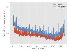
**Fig. 11.** Sum of the 1-norm distance between commands from both MARL and integrator controllers and the result of direct projection of the phase onto  $B_{tt}$  modes over 1000 frames. Tip-tilt is not included. As only 1262 modes are controlled through MARL, the last 21 modes are either controller by an integrator approach (16 modes) or discarded low sensitivity modes (5 modes) that is why both integrator and MARL have the same error on those.
