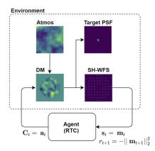
Fig. 1. Agent-environment interaction with a direct RL approach. The environment corresponds to the atmosphere, the DM and the WFS while the agent corresponds to the RTC.
