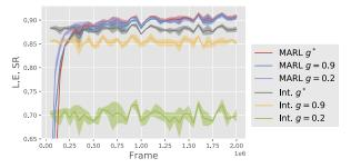
**Fig. 7.** Comparison of L.E. SR obtained in the evaluation episodes for MARL and integrator controllers for different values of integrator gain. The optimal gain is g = 0.7 and is denoted with an asterisk.
