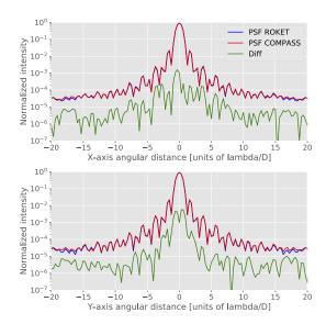
**Fig. 9.** COMPASS and ROKET reconstructions of the PSF with the MARL controller after 20000 frames. The green curve shows the difference in value between both PSF's. The L.E. SR is 0.918 in the case of ROKET and 0.919 in the case of COMPASS.
