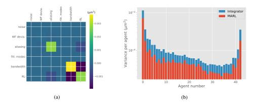
**Fig. 10.** a) Covariance of all the error terms in the current simulation: no noise, wind direction profile 1 and wind speed profile 2. b) Summed variance of modes controlled by a given agent (y axis in log-scale). The last agent controls tip-tilt. Other agents control 30 modes each and are ordered from lower order modes to higher order modes.
