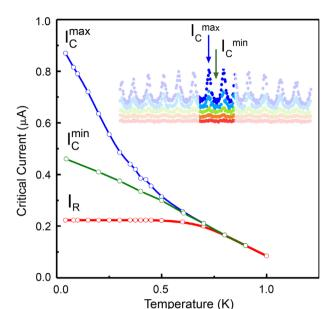
**Figure 3.** Evolution of critical currents with temperature. Blue curve: evolution of the maximum critical current (measured at the first peak at H=0 Oe). Green curve: evolution of the minimum current (first minimum, at  $H\simeq0.5$  Oe). Red line: retrapping current.
